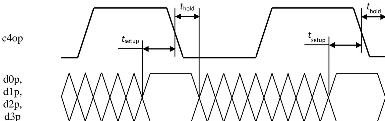
Fig. 2. Input Data Alignment to Output  $c4$  Clock
