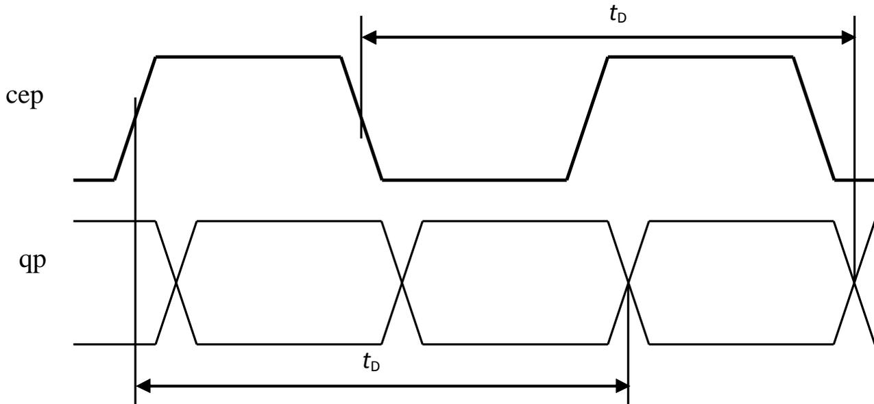
Fig. 3. Output Data to Input Clock Delay
