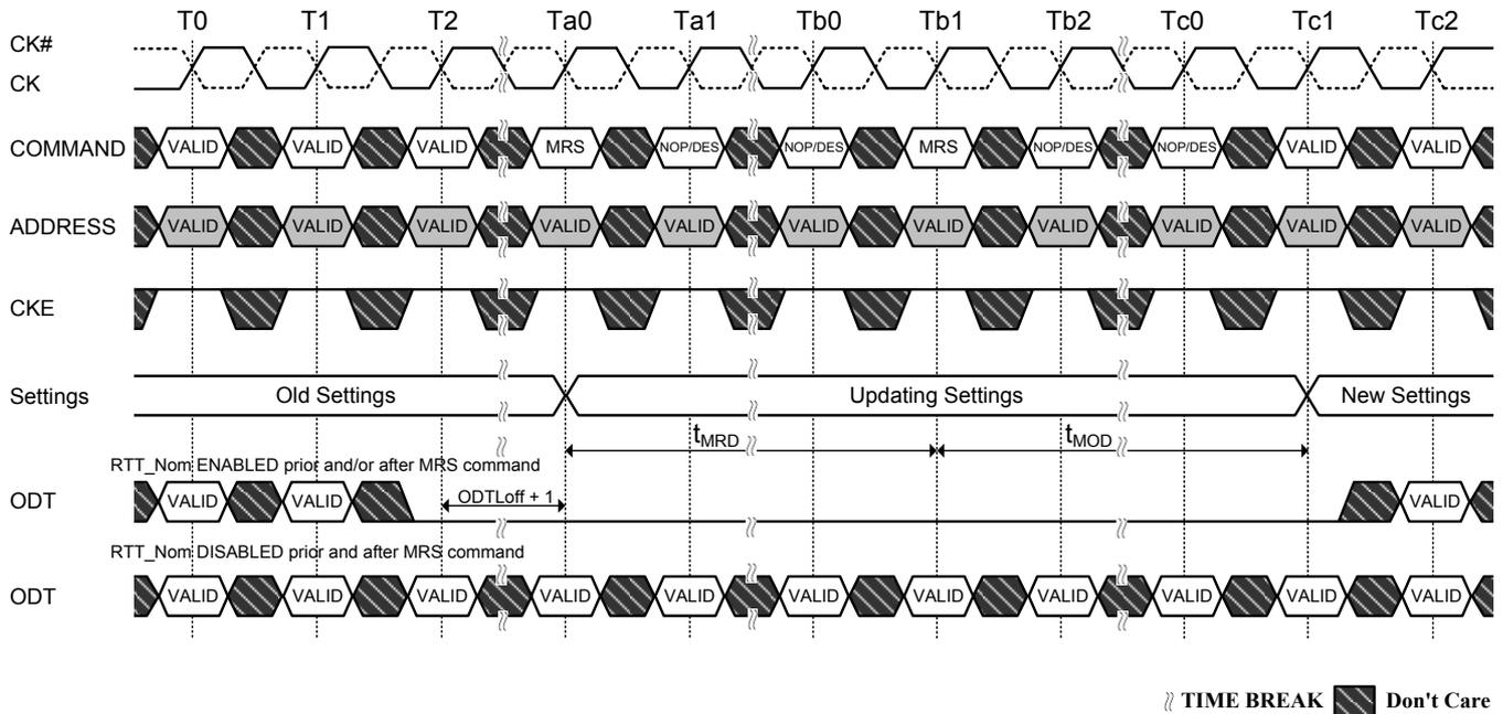
The MRS command to Non-MRS command delay,  $t_{MOD}$ , is required for the DRAM to update the features except DLL reset, and is the minimum time required from an MRS command to a non-MRS command excluding NOP and DES shown in Figure of  $t_{MOD}$  timing.
