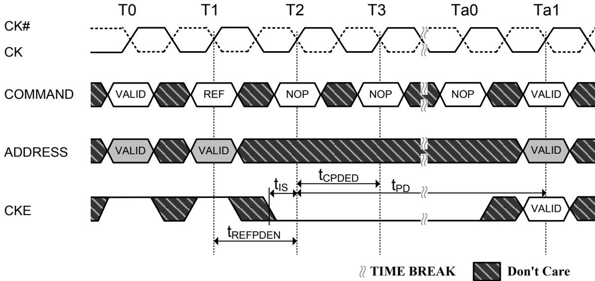
**Figure 62. Active Command to Power-Down Entry**
