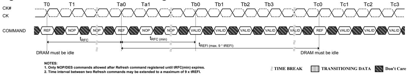
**Figure 54. Self-Refresh Entry/Exit Timing**
