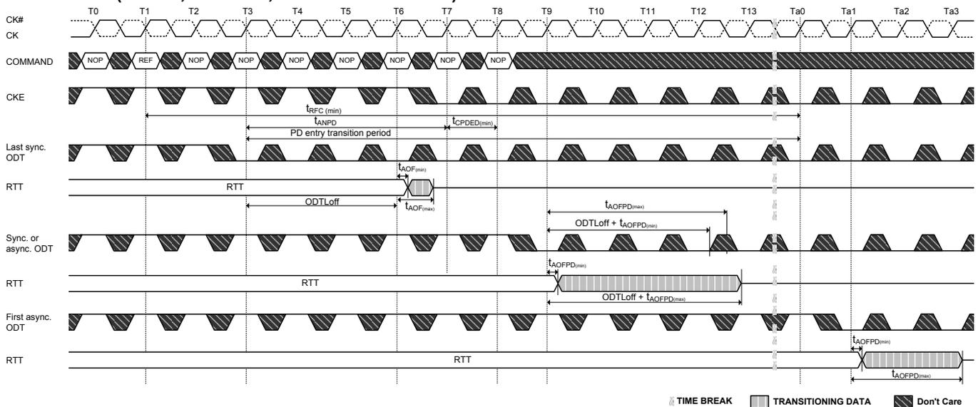
**Figure 75. Asynchronous to synchronous transition during Precharge Power Down**
