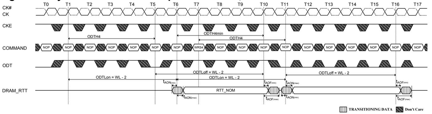
**Figure 67. Dynamic ODT Behavior with ODT being asserted before and after the write**
