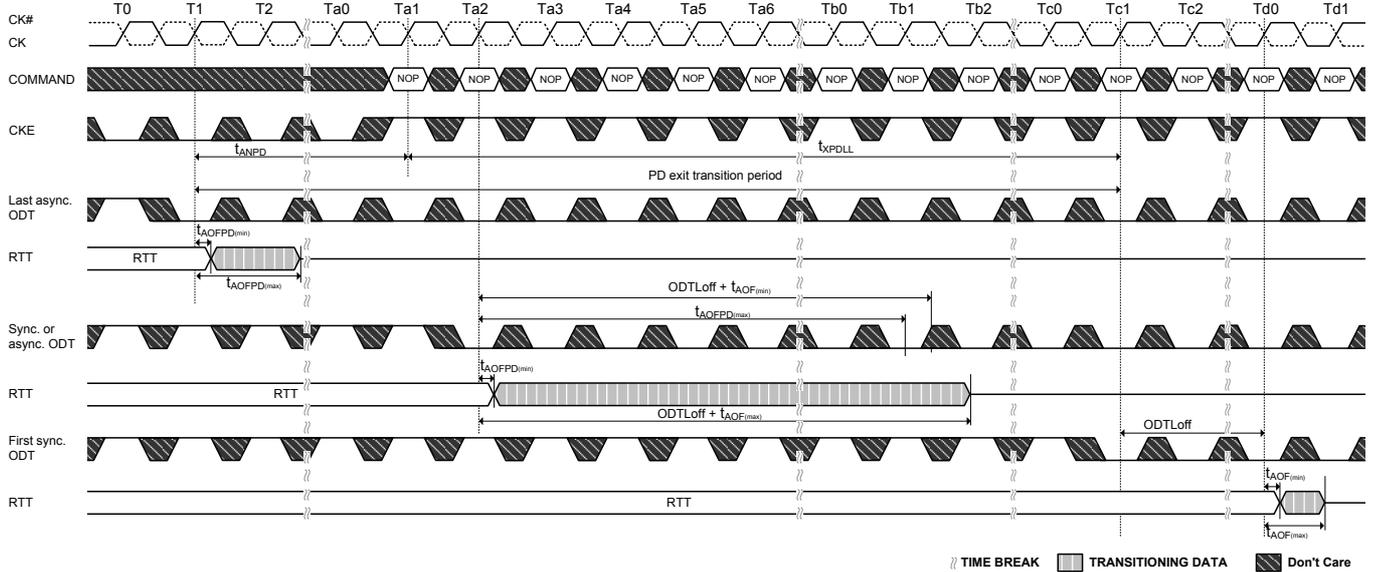
**Figure 76. Transition period for short CKE cycles, entry and exit period overlapping**
