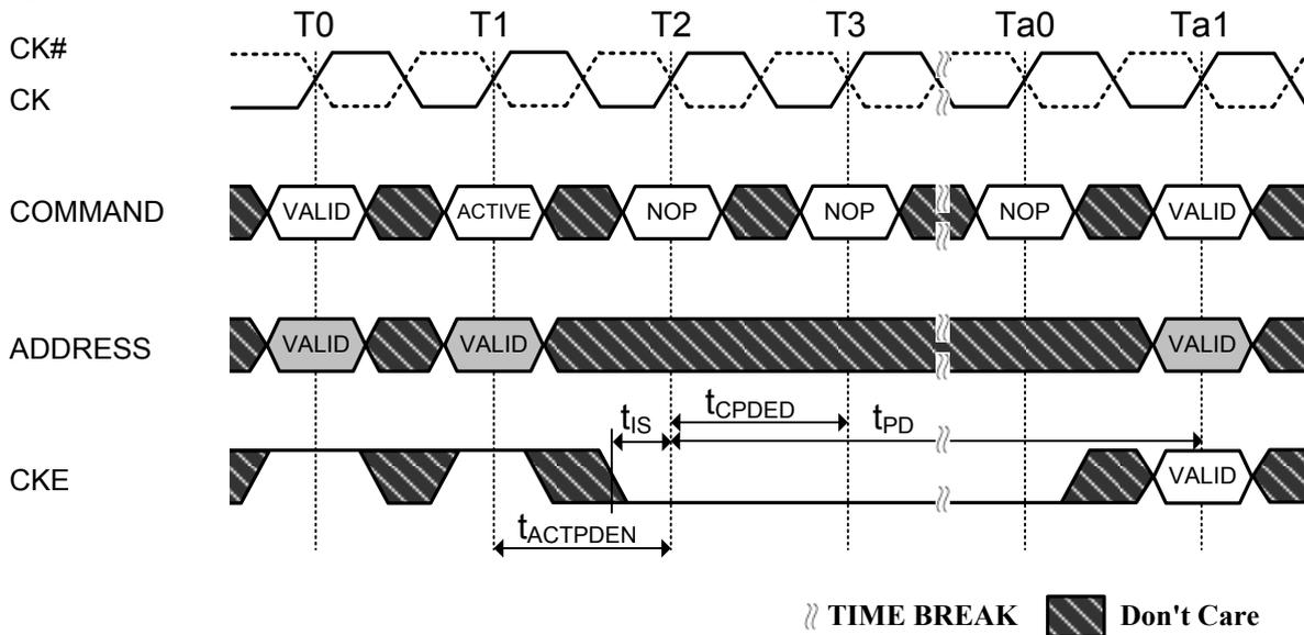
**Figure 63. Precharge, Precharge all command to Power-Down Entry**
