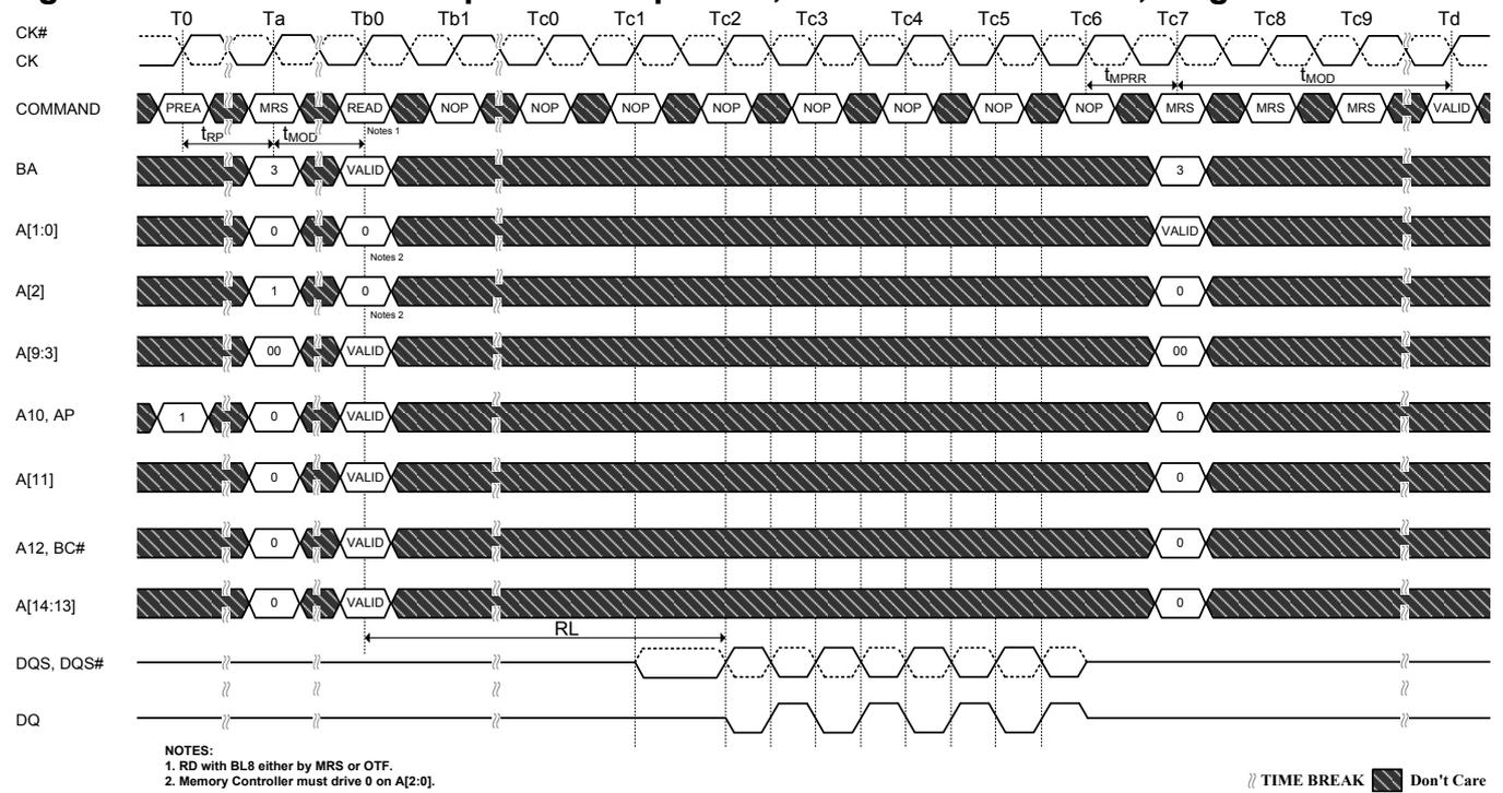
**Figure 26. MPR Readout of predefined pattern, BL8 fixed burst order, back to back radout**
