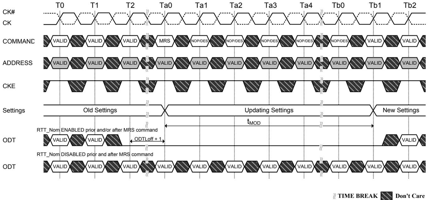
The mode register contents can be changed using the same command and timing requirements during normal operation as long as the DRAM is in idle state, i.e., all banks are in the precharged state with  $t_{RP}$  satisfied, all data bursts are completed and CKE is high prior to writing into the mode register. The mode registers are divided into various fields depending on the functionality and/or modes.
