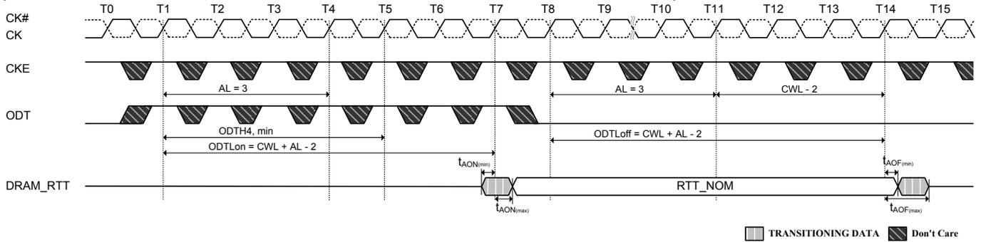
**Figure 66. Synchronous ODT example with BL = 4, WL = 7**
