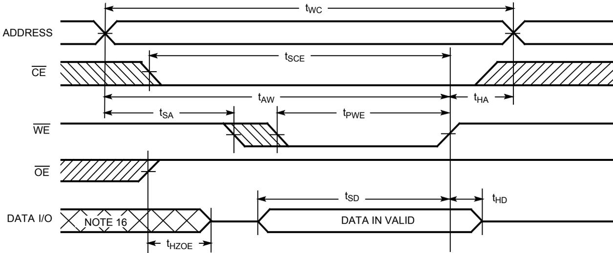
Figure 7. Write Cycle No. 2 ( $\overline{WE}$  Controlled,  $\overline{OE}$  Low)<sup>[15, 17]</sup>
