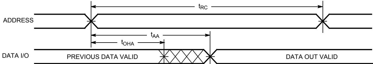
Figure 5. Read Cycle No. 2 ( $\overline{OE}$  Controlled)<sup>[12, 13]</sup>
