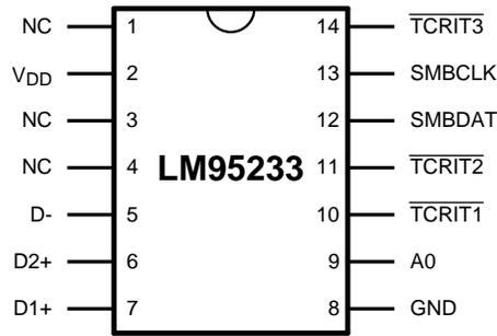
Figure 1. 14-Lead WSON - TOP VIEW
