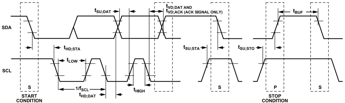
**Figure 2. I<sup>2</sup>C Port Timing Diagram**
