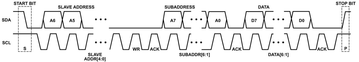
Figure 64. I<sup>2</sup>C Data Transfer Timing
