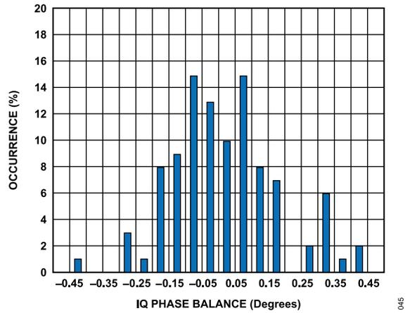
Figure 45. IQ Phase Balance, Narrow-Band Mode, Nominal Conditions
