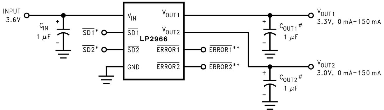
\*SD1 and SD2 must be actively terminated through a pull up resistor. Tie to V<sub>IN</sub> if not used.
