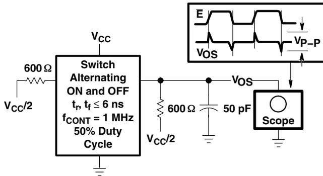
Figure 5. Control to Switch Feedthrough Noise Test Circuit
