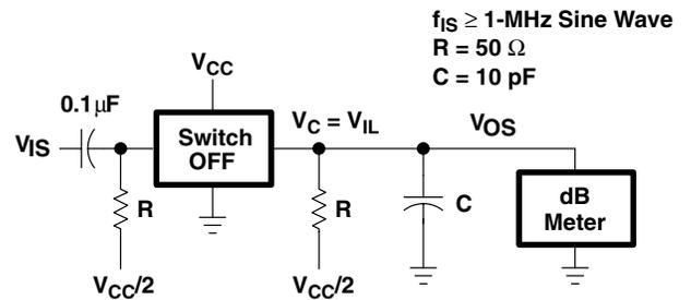
Figure 6. Switch OFF Signal Feedthrough Test Circuit
