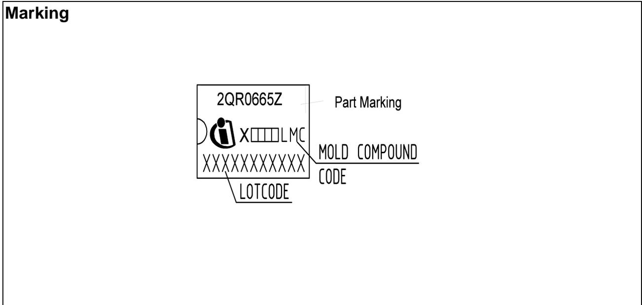
Figure 15 Marking for ICE2QR0665Z
