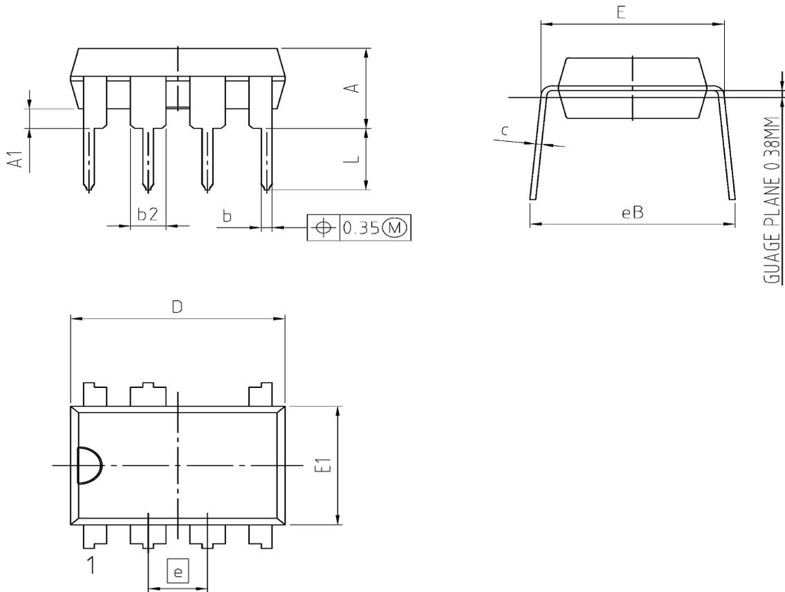
1) DOES NOT INCLUDE MOLD FLASH OR PROTRUSIONS.
