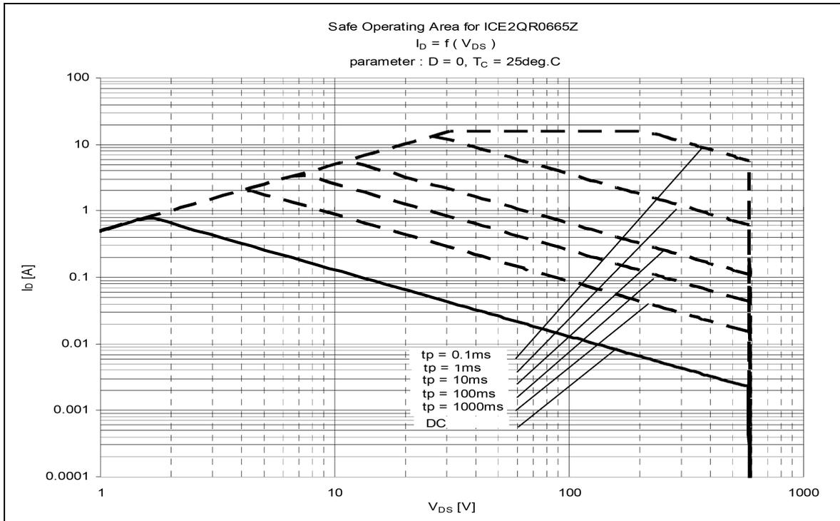
Figure 9 Safe Operating Area(SOA) curve for ICE2QR0665Z
