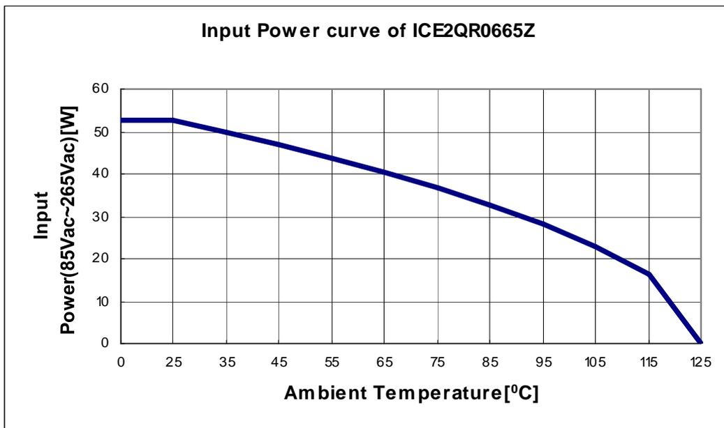
Figure 12 Input Power curve  $V_{in}=85\sim 265\text{Vac}; P_{in}=f(T_a)$
