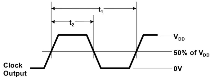
Figure 6. Rise Time =  $T_{RF}$  Fall Time =  $T_{RF}$
