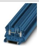
Disconnect terminal block, Connection type: Screw connection, Cross section: 0.14 mm² - 4 mm², AWG: 26 - 12, Nominal current: 20 A, Nominal voltage: 400 V, Length: 57.8 mm, Width: 5.2 mm, Color: blue, Assembly: NS 35/7,5, NS 35/15
