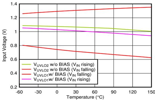
Figure 6-83.  $V_{IN}$  UVLO vs Temperature
