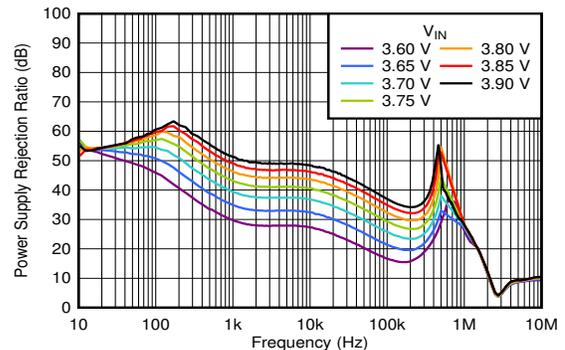
$I_{OUT} = 3\text{ A}$ ,  $C_{OUT} = 47\text{ }\mu\text{F} \parallel 10\text{ }\mu\text{F} \parallel 10\text{ }\mu\text{F}$ ,  $C_{NR/SS} = 10\text{ nF}$ ,
