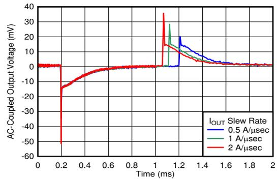
$V_{OUT} = 5\text{ V}$ ,  $I_{OUT,DC} = 100\text{ mA}$ ,  $I_{OUT} = 100\text{ mA}$  to  $3\text{ A}$ ,
