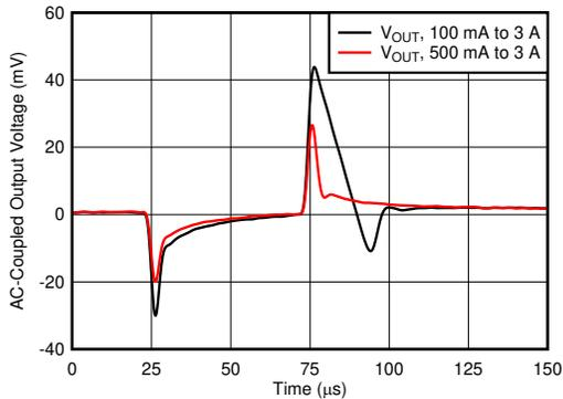
$V_{IN} = 1.2\text{ V}$ ,  $V_{BIAS} = 5\text{ V}$ ,  $C_{OUT} = 47\text{ }\mu\text{F} \parallel 10\text{ }\mu\text{F} \parallel 10\text{ }\mu\text{F}$ ,  $V_{OUT} = 0.9\text{ V}$ ,  $C_{NR/SS} = C_{FF} = 10\text{ nF}$ , slew rate =  $1\text{ A}/\mu\text{s}$
