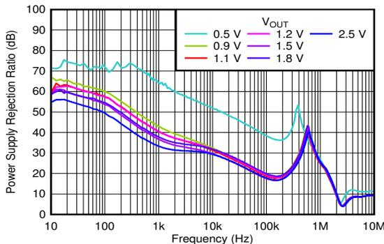
$V_{IN} = V_{OUT} + 0.3\text{ V}$  or  $V_{IN} = 1.1\text{ V}$  (whichever is greater),  $V_{BIAS} = 5\text{ V}$ ,  $I_{OUT} = 3\text{ A}$ ,  $C_{OUT} = 47\text{ }\mu\text{F} \parallel 10\text{ }\mu\text{F} \parallel 10\text{ }\mu\text{F}$ ,
