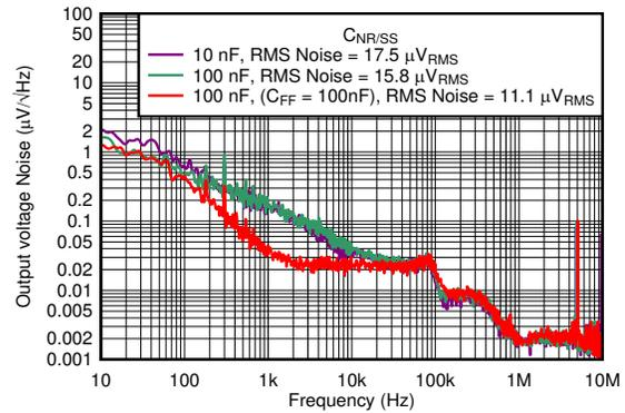
$V_{IN} = V_{OUT} + 0.3\text{ V}$ ,  $V_{BIAS} = 5\text{ V}$ ,  $I_{OUT} = 3\text{ A}$ ,  $C_{OUT} = 47\text{ }\mu\text{F} \parallel 10\text{ }\mu\text{F} \parallel 10\text{ }\mu\text{F}$ ,  $C_{FF} = 10\text{ nF}$ , RMS noise BW = 10 Hz to 100 kHz
