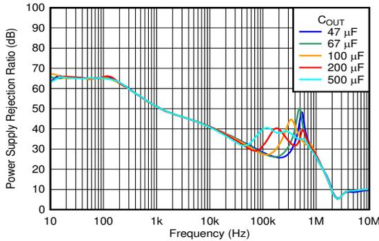
$V_{IN} = 1.4\text{ V}$ ,  $V_{BIAS} = 5\text{ V}$ ,  $V_{OUT} = 1\text{ V}$ ,  $I_{OUT} = 3\text{ A}$ ,
