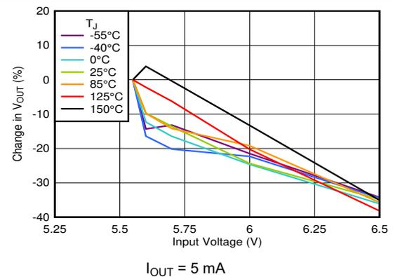
Figure 6-77. Line Regulation vs  $V_{IN}$  (5.15-V Output)
