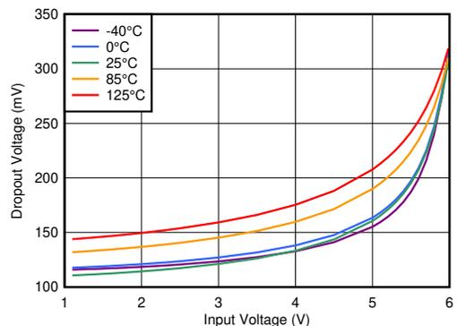
$I_{OUT} = 3\text{ A}$ ,  $V_{BIAS} = 6.5\text{ V}$
