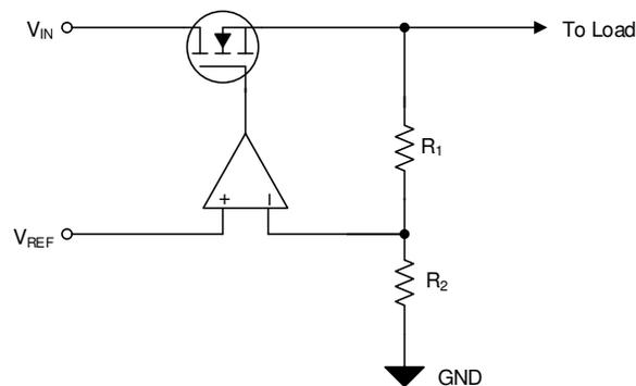
$$V_{OUT} = V_{REF} \times (1 + R_1 / R_2).$$
