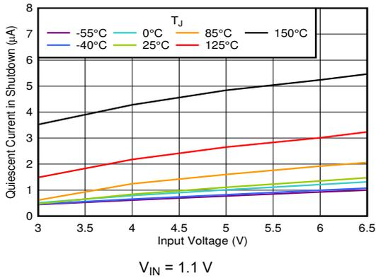
Figure 6-81. Shutdown Current vs  $V_{IN}$  With Bias
