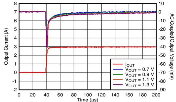
$V_{IN} = V_{OUT} + 0.5\text{ V}$ ,  $V_{BIAS} = 5\text{ V}$ ,  $I_{OUT} = 100\text{ mA}$  to  $3\text{ A}$ , slew rate =  $1\text{ A}/\mu\text{s}$ ,  $C_{NR/SS} = C_{FF} = 10\text{ nF}$ ,  $C_{OUT} = 47\text{ }\mu\text{F} \parallel 10\text{ }\mu\text{F} \parallel 10\text{ }\mu\text{F}$
