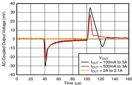
$V_{IN} = 1.2\text{ V}$ ,  $V_{OUT} = 0.7\text{ V}$ ,  $V_{BIAS} = 5\text{ V}$ , slew rate =  $1\text{ A}/\mu\text{s}$ ,
