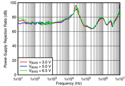
$V_{IN} = V_{OUT} + 0.3\text{ V}$ ,  $V_{OUT} = 1\text{ V}$ ,  $I_{OUT} = 3\text{ A}$ ,  $C_{OUT} = 47\text{ }\mu\text{F} \parallel 10\text{ }\mu\text{F} \parallel 10\text{ }\mu\text{F}$ ,  $C_{NR/SS} = 10\text{ nF}$ ,  $C_{FF} = 10\text{ nF}$
