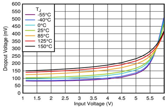
$I_{OUT} = 3\text{ A}$ ,  $V_{BIAS} = 5.0\text{ V}$
