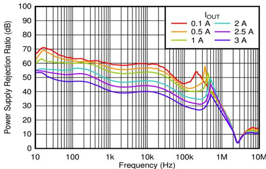
$V_{IN} = 5.5\text{ V}$ ,  $V_{OUT} = 5\text{ V}$ ,  $I_{OUT} = 3\text{ A}$ ,  $C_{OUT} = 47\text{ }\mu\text{F} \parallel 10\text{ }\mu\text{F} \parallel 10\text{ }\mu\text{F}$  ||
