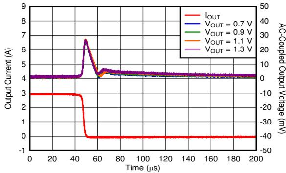
$V_{IN} = V_{OUT} + 0.5\text{ V}$ ,  $V_{BIAS} = 5\text{ V}$ ,  $I_{OUT} = 3\text{ A}$  to  $100\text{ mA}$ ,
