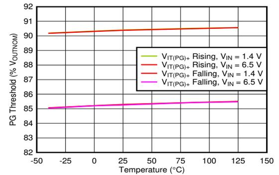
**Figure 6-88. PG Threshold vs Temperature**
