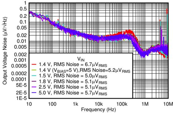
$V_{OUT} = 0.7\text{ V}$ ,  $I_{OUT} = 3\text{ A}$ ,  $C_{OUT} = 47\text{ }\mu\text{F} \parallel 10\text{ }\mu\text{F} \parallel 10\text{ }\mu\text{F}$ ,  $C_{NR/SS} = 10\text{ nF}$ ,  $C_{FF} = 10\text{ nF}$ , RMS noise BW = 10 Hz to 100 kHz
