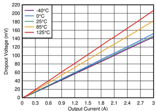
$V_{IN} = 1.4\text{ V}$
