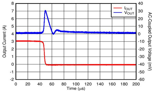
$V_{IN} = V_{OUT} + 0.5\text{ V}$ ,  $V_{OUT} = 0.7\text{ V}$ ,  $I_{OUT} = 3\text{ A}$  to  $100\text{ mA}$ ,
