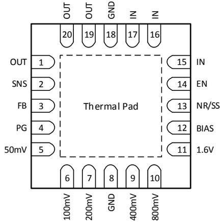
Figure 5-1. RGR Package (TPS7A8400A), 20-Pin VQFN, Top View
