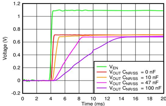
$V_{IN} = 1.2\text{ V}$ ,  $V_{OUT} = 0.7\text{ V}$ ,  $V_{BIAS} = 5\text{ V}$ ,  $I_{OUT} = 3\text{ A}$ ,  $C_{OUT} = 47\text{ }\mu\text{F} \parallel 10\text{ }\mu\text{F} \parallel 10\text{ }\mu\text{F}$ ,  $C_{FF} = 10\text{ nF}$
