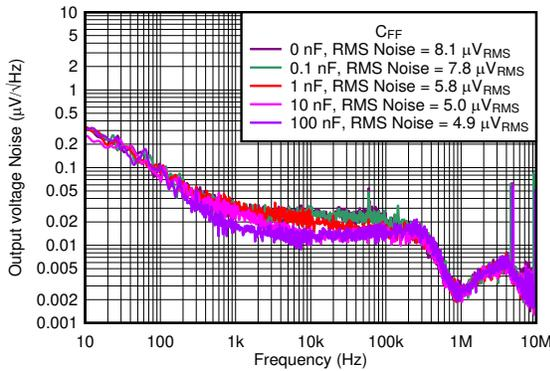
$V_{OUT} = 0.7\text{ V}$ ,  $V_{IN} = 1.1\text{ V}$ ,  $V_{BIAS} = 5\text{ V}$ ,  $I_{OUT} = 3\text{ A}$ ,  $C_{OUT} = 47\text{ }\mu\text{F} \parallel 10\text{ }\mu\text{F} \parallel 10\text{ }\mu\text{F}$ ,  $C_{NR/SS} = 10\text{ nF}$ , RMS noise BW = 10 Hz to 100 kHz
