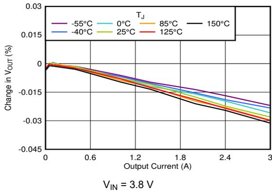
Figure 6-73. Load Regulation vs  $I_{OUT}$  (3.3-V Output)
