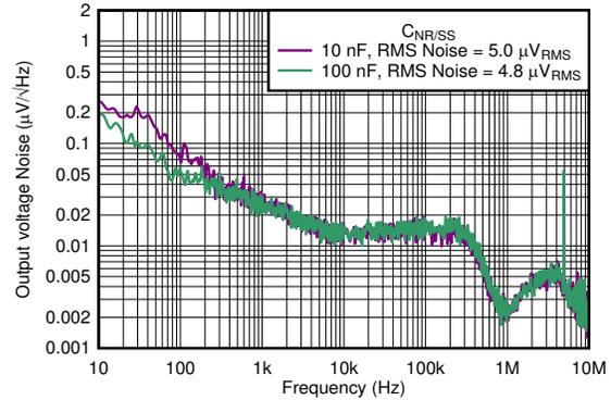
$V_{OUT} = 0.7\text{ V}$ ,  $V_{IN} = 1.1\text{ V}$ ,  $V_{BIAS} = 5\text{ V}$ ,  $I_{OUT} = 3\text{ A}$ ,  $C_{OUT} = 47\text{ }\mu\text{F} \parallel 10\text{ }\mu\text{F} \parallel 10\text{ }\mu\text{F}$ ,  $C_{FF} = 10\text{ nF}$ , RMS noise BW = 10 Hz to 100 kHz
