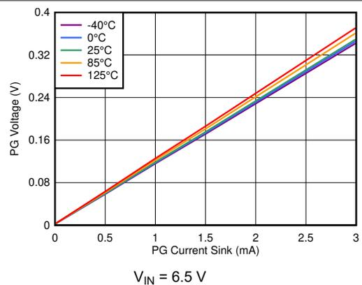
Figure 6-41. PG Voltage vs PG Current Sink
