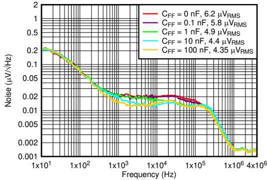
$V_{IN} = V_{OUT} + 0.3\text{ V}$ ,  $V_{BIAS} = 5\text{ V}$ ,  $I_{OUT} = 3\text{ A}$ ,  $C_{OUT} = 47\text{ }\mu\text{F} \parallel 10\text{ }\mu\text{F} \parallel 10\text{ }\mu\text{F}$ ,  $C_{NR/SS} = 10\text{ nF}$ , RMS noise BW = 10 Hz to 100 kHz
