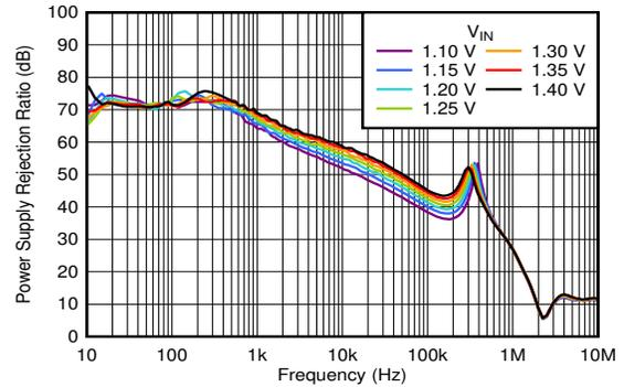
$I_{OUT} = 3\text{ A}$ ,  $V_{BIAS} = 5\text{ V}$ ,  $C_{OUT} = 47\text{ }\mu\text{F} \parallel 10\text{ }\mu\text{F} \parallel 10\text{ }\mu\text{F}$ ,
