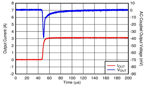
$V_{IN} = V_{OUT} + 0.5\text{ V}$ ,  $V_{OUT} = 0.7\text{ V}$ ,  $I_{OUT} = 100\text{ mA}$  to  $3\text{ A}$ ,
