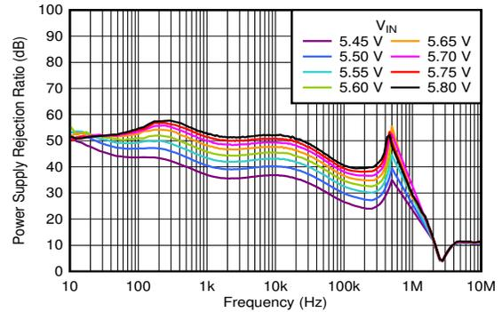
$V_{OUT} = 5\text{ V}$ ,  $I_{OUT} = 3\text{ A}$ ,  $C_{OUT} = 47\text{ }\mu\text{F} \parallel 10\text{ }\mu\text{F} \parallel 10\text{ }\mu\text{F}$ ,
