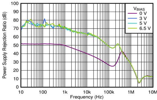
$V_{IN} = 1.4\text{ V}$ ,  $I_{OUT} = 1\text{ A}$ ,  $C_{OUT} = 47\text{ }\mu\text{F} \parallel 10\text{ }\mu\text{F} \parallel 10\text{ }\mu\text{F}$ ,
