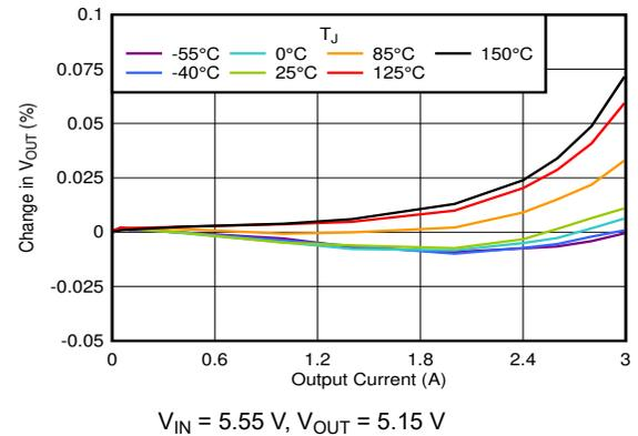
Figure 6-74. Load Regulation vs  $I_{OUT}$  (5-V Output)
