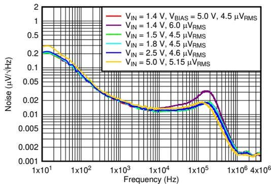
$I_{OUT} = 3\text{ A}$ ,  $C_{OUT} = 47\text{ }\mu\text{F} \parallel 10\text{ }\mu\text{F} \parallel 10\text{ }\mu\text{F}$ ,  $C_{NR/SS} = 10\text{ nF}$ ,
