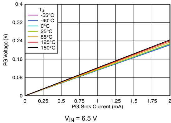
**Figure 6-87. PG Voltage vs PG Current Sink**
