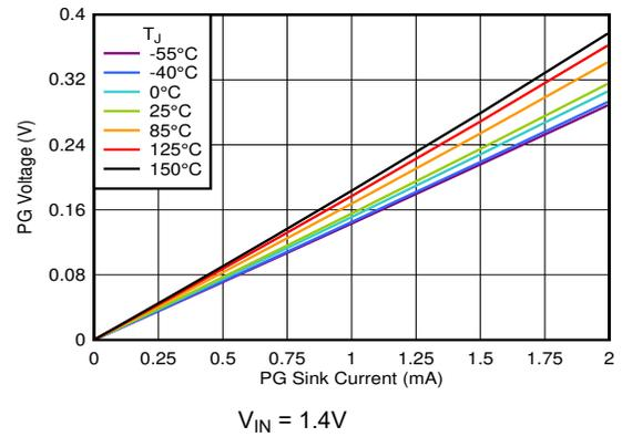
**Figure 6-86. PG Voltage vs PG Current Sink**
