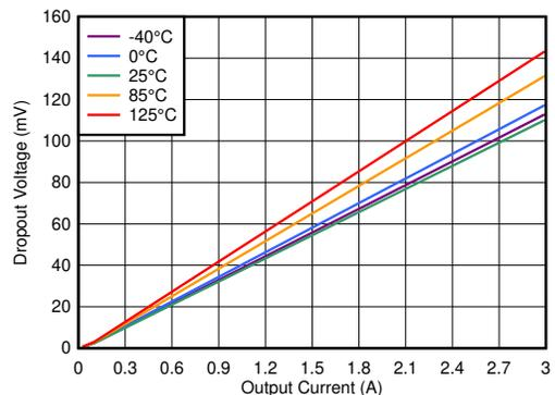
$V_{IN} = 1.1\text{ V}$ ,  $V_{BIAS} = 3\text{ V}$
