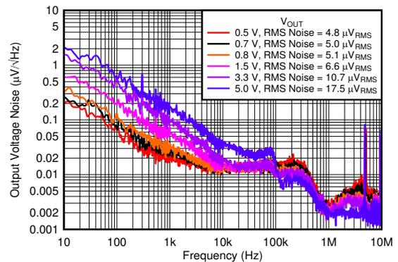
$V_{IN} = V_{OUT} + 0.3\text{ V}$  or  $V_{IN} = 1.1\text{ V}$  (whichever is greater),  $V_{BIAS} = 5\text{ V}$  for  $V_{IN} \leq 2.2\text{ V}$ ,  $I_{OUT} = 3\text{ A}$ ,  $C_{OUT} = 47\text{ }\mu\text{F} \parallel 10\text{ }\mu\text{F} \parallel 10\text{ }\mu\text{F}$ ,  $C_{NR/SS} = 10\text{ nF}$ ,  $C_{FF} = 10\text{ nF}$ , RMS noise BW =  $10\text{ Hz}$  to  $100\text{ kHz}$
