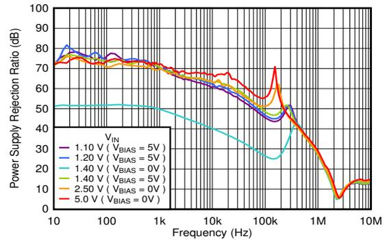
$I_{OUT} = 1\text{ A}$ ,  $C_{OUT} = 47\text{ }\mu\text{F} \parallel 10\text{ }\mu\text{F} \parallel 10\text{ }\mu\text{F}$ ,  $C_{NR/SS} = 10\text{ nF}$ ,
