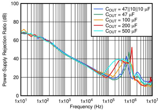
$V_{IN} = 1.4\text{ V}$ ,  $V_{BIAS} = 5\text{ V}$ ,  $V_{OUT} = 1\text{ V}$ ,  $I_{OUT} = 3\text{ A}$ ,
