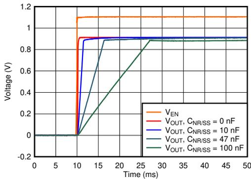
$V_{IN} = 1.2\text{ V}$ ,  $V_{OUT} = 0.9\text{ V}$ ,  $V_{BIAS} = 5\text{ V}$ ,  $I_{OUT} = 3\text{ A}$ ,  $C_{OUT} = 47\text{ }\mu\text{F} \parallel 10\text{ }\mu\text{F} \parallel 10\text{ }\mu\text{F}$ ,  $C_{FF} = 10\text{ nF}$
