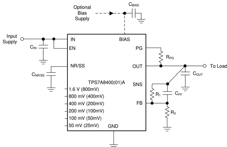
**Figure 8-1. Adjustable Operation**
