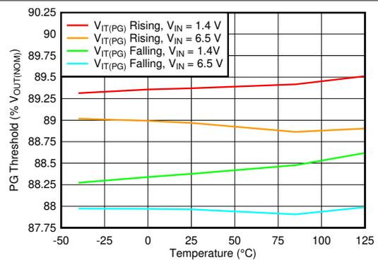
Figure 6-42. PG Threshold vs Temperature
