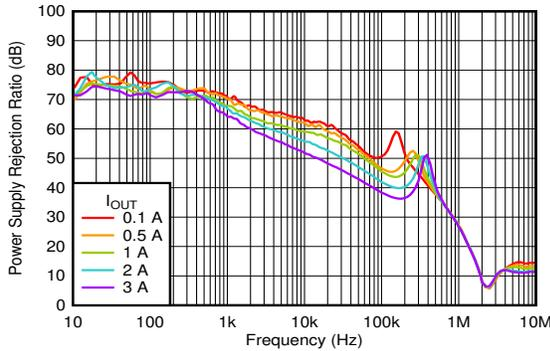
$V_{IN} = 1.1\text{ V}$ ,  $V_{BIAS} = 5\text{ V}$ ,  $C_{OUT} = 47\text{ }\mu\text{F} \parallel 10\text{ }\mu\text{F} \parallel 10\text{ }\mu\text{F}$ ,
