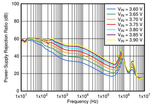
$I_{OUT} = 3\text{ A}$ ,  $C_{OUT} = 47\text{ }\mu\text{F} \parallel 10\text{ }\mu\text{F} \parallel 10\text{ }\mu\text{F}$ ,
