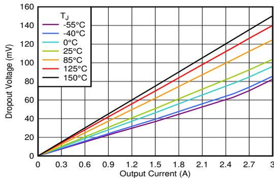
$V_{IN} = 1.1\text{ V}$ ,  $V_{BIAS} = 5.0\text{ V}$
