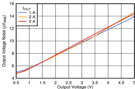
$V_{IN} = V_{OUT} + 0.3\text{ V}$  or  $V_{IN} = 1.1\text{ V}$  (whichever is greater),  $V_{BIAS} = 5\text{ V}$  for  $V_{IN} \leq 2.2\text{ V}$ ,  $C_{OUT} = 47\text{ }\mu\text{F} \parallel 10\text{ }\mu\text{F} \parallel 10\text{ }\mu\text{F}$ ,  $C_{NR/SS} = 10\text{ nF}$ ,  $C_{FF} = 10\text{ nF}$ , RMS noise BW =  $10\text{ Hz}$  to  $100\text{ kHz}$
