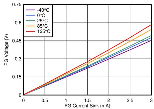
Figure 6-40. PG Voltage vs PG Current Sink
