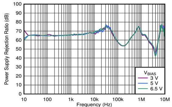
$V_{IN} = V_{OUT} + 0.3\text{ V}$ ,  $V_{OUT} = 1\text{ V}$ ,  $I_{OUT} = 3\text{ A}$ ,  $C_{OUT} = 47\text{ }\mu\text{F} \parallel 10\text{ }\mu\text{F} \parallel 10\text{ }\mu\text{F}$  ||
