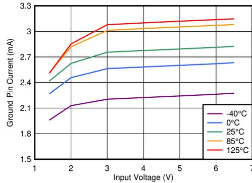
$V_{BIAS} = 0\text{ V}$ ,  $I_{OUT} = 5\text{ mA}$
