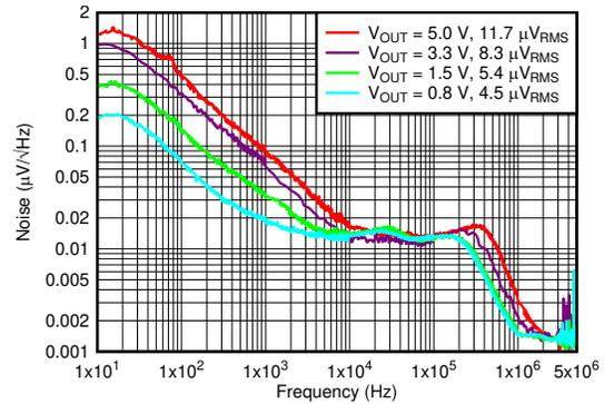
$V_{IN} = V_{OUT} + 0.3\text{ V}$  and  $V_{BIAS} = 5\text{ V}$  for  $V_{OUT} \leq 2.2\text{ V}$ ,  $I_{OUT} = 3\text{ A}$ ,  $C_{OUT} = 47\text{ }\mu\text{F} \parallel 10\text{ }\mu\text{F} \parallel 10\text{ }\mu\text{F}$ ,  $C_{NR/SS} = 10\text{ nF}$ ,  $C_{FF} = 10\text{ nF}$ , RMS noise BW =  $10\text{ Hz}$  to  $100\text{ kHz}$
