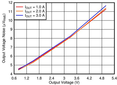
$V_{IN} = V_{OUT} + 0.3\text{ V}$  and  $V_{BIAS} = 5\text{ V}$  for  $V_{OUT} \leq 2.2\text{ V}$ ,
