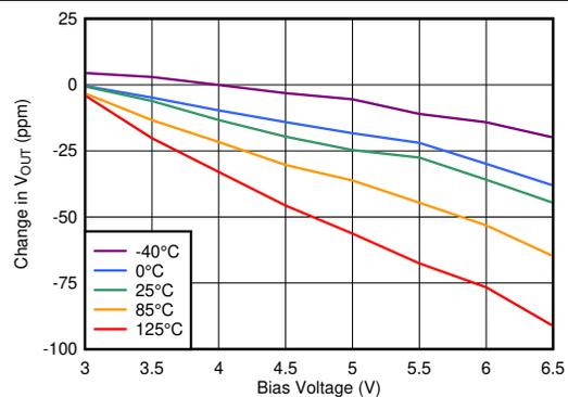
$V_{OUT} = 0.8\text{ V}$ ,  $V_{IN} = 1.1\text{ V}$ ,  $I_{OUT} = 5\text{ mA}$ ,  $V_{BIAS} = 5\text{ V}$
