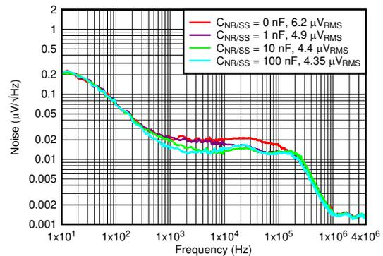
$V_{IN} = V_{OUT} + 0.3\text{ V}$ ,  $V_{BIAS} = 5\text{ V}$ ,  $I_{OUT} = 3\text{ A}$ ,  $C_{OUT} = 47\text{ }\mu\text{F} \parallel 10\text{ }\mu\text{F} \parallel 10\text{ }\mu\text{F}$ ,  $C_{FF} = 10\text{ nF}$ , RMS noise BW =  $10\text{ Hz}$  to  $100\text{ kHz}$
