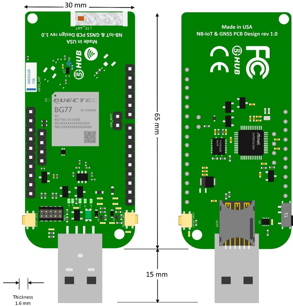
Figure 3. Physical Characteristics.
