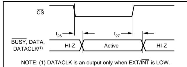
FIGURE 9. Enable and Disable Timing for Digital Outputs.
