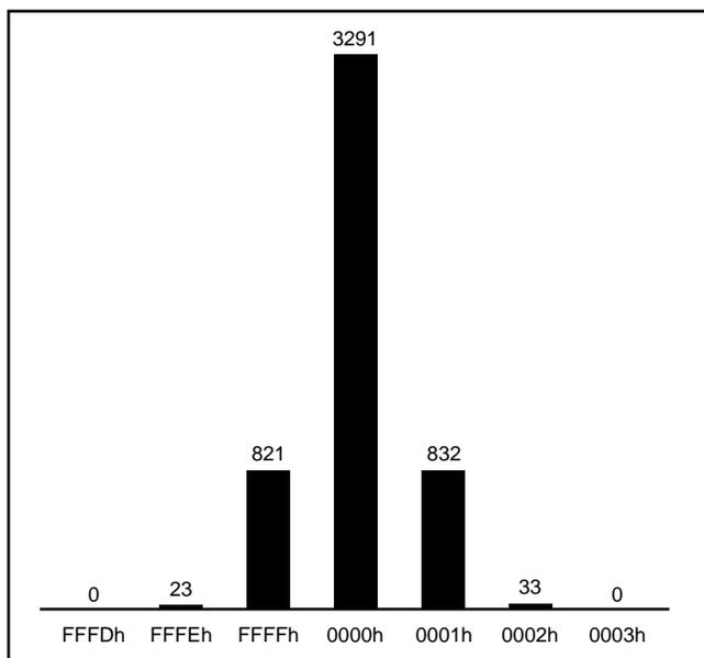
FIGURE 14. Histogram of 5,000 Conversions with Input Grounded.
