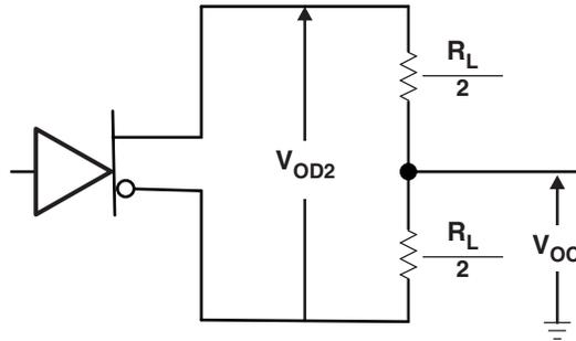
Figure 1. Driver Test Circuit,  $V_{OD}$  and  $V_{OC}$
