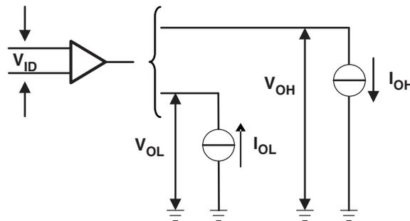
Figure 2. Receiver Test Circuit,  $V_{OH}$  and  $V_{OL}$
