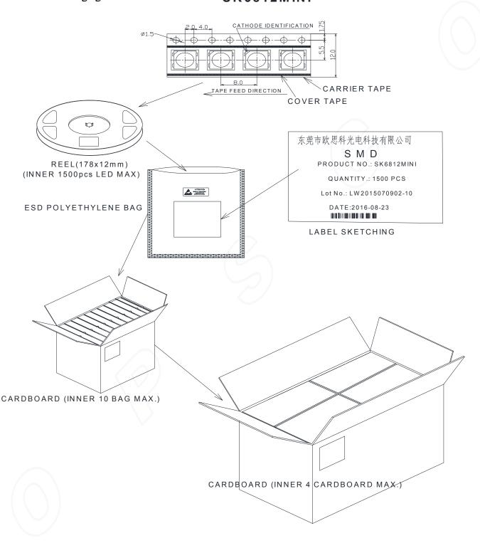
The reel pack is applied in SMD LED. The LEDs are packed in cardboard boxes after packaging in normal or antielectrostatic bags. cardboard boxes will be used to protect the LEDs from mechanical shocks during transportation. The boxes are not water resistant and therefore must be kept away from water and moisture.
