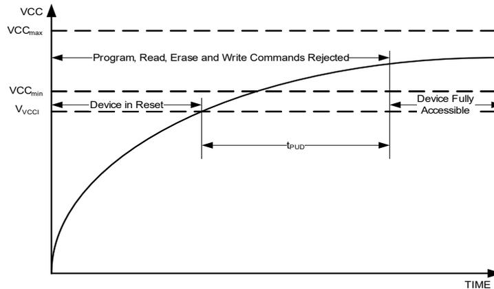
Power up delay  $t_{PUD}$  is based on  $V_{CCI}$  which is the voltage level at which the internal reset circuit releases and signals the controller to initiate the power-on reset condition for a 75 $\mu$ s maximum period.
