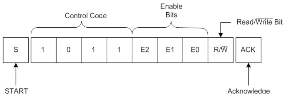
Upon receiving the correct Control Code, the chip enable bits, and the  $\overline{R/W}$  bit, the device performs an acknowledge by pulling the SDA line low during the 9th clock pulse. As stated above, the device will now be set for either a read or a write operation by the  $\overline{R/W}$  bit.
