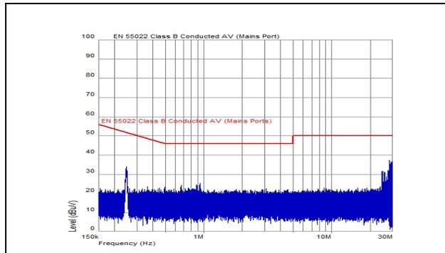
EMI with filter @  $V_i = 48 V$ , max  $I_o$ .
