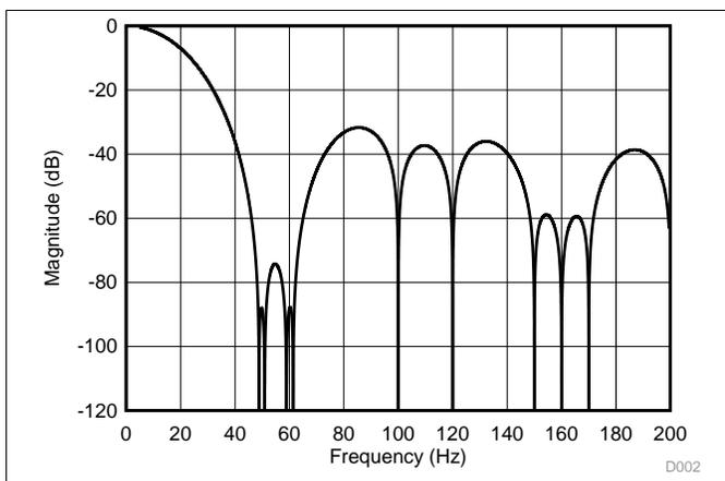
**Figure 45. Filter Response (Normal Mode, DR = 20 SPS)**
