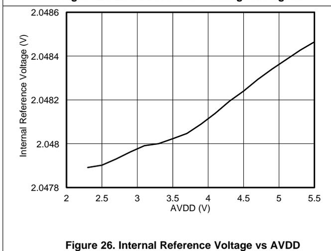
Figure 26. Internal Reference Voltage vs AVDD
