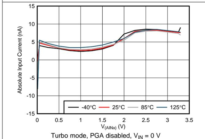
Figure 6. Absolute Input Current vs Absolute Input Voltage
