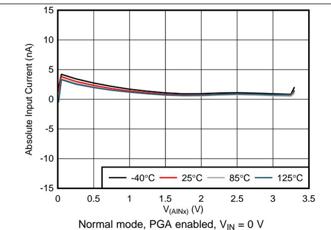
Figure 5. Absolute Input Current vs Absolute Input Voltage
