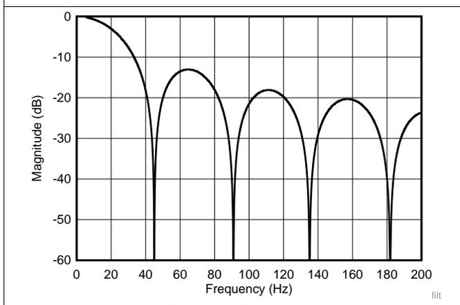
**Figure 47. Filter Response (Normal Mode, DR = 45 SPS)**
