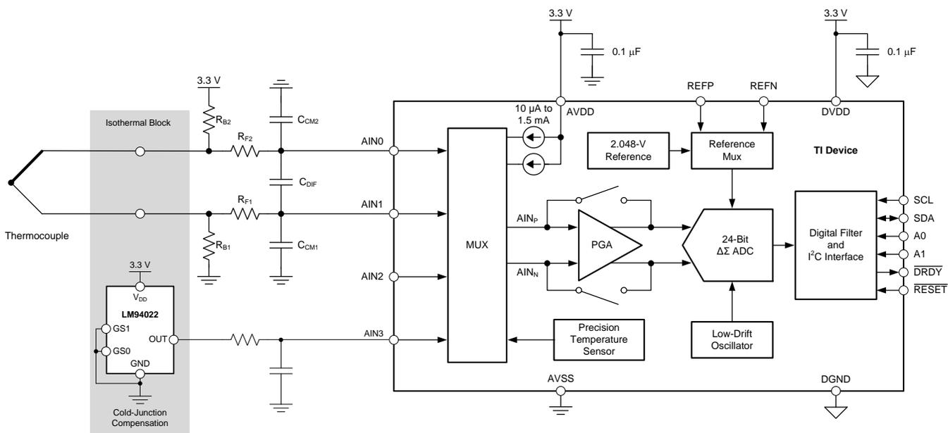
Figure 71. Thermocouple Measurement
