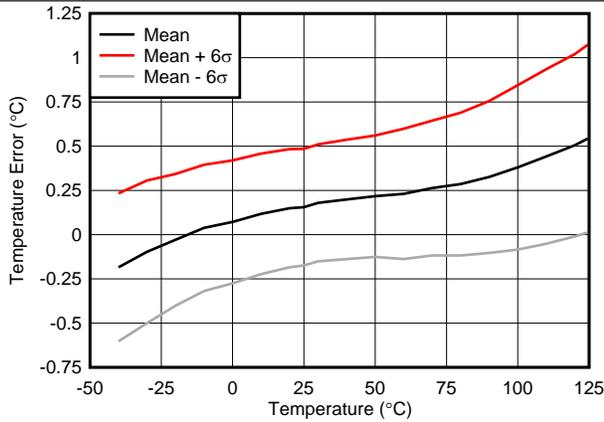
**Figure 34. Internal Temperature Sensor Accuracy vs Temperature**
