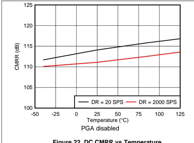
Figure 22. DC CMRR vs Temperature
