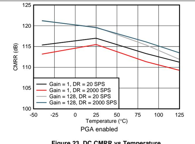
Figure 23. DC CMRR vs Temperature
