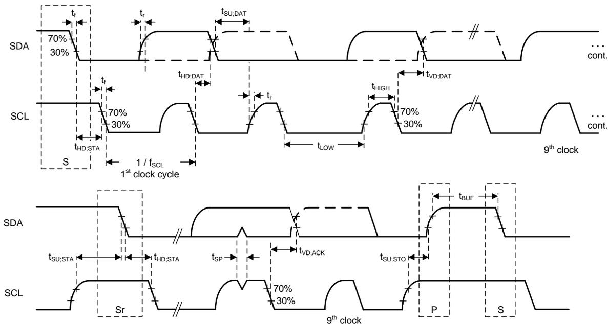
Figure 1. I<sup>2</sup>C Timing Requirements
