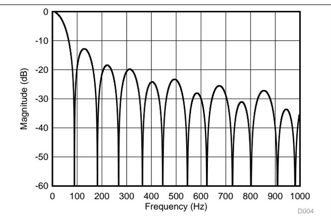
**Figure 48. Filter Response (Normal Mode, DR = 90 SPS)**
