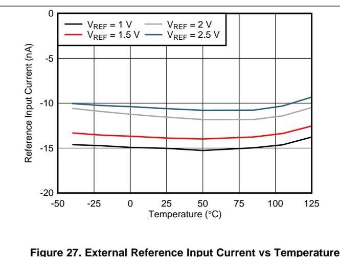
Figure 27. External Reference Input Current vs Temperature
