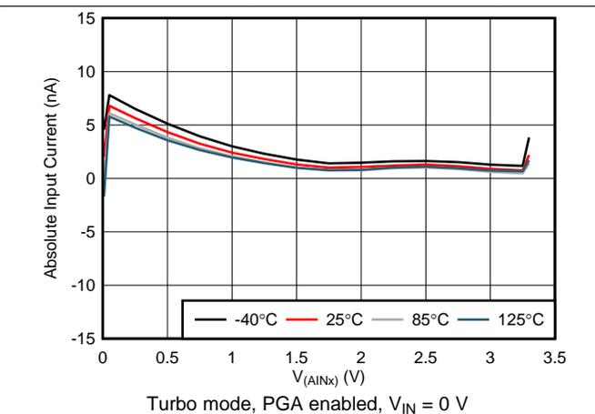
Figure 7. Absolute Input Current vs Absolute Input Voltage
