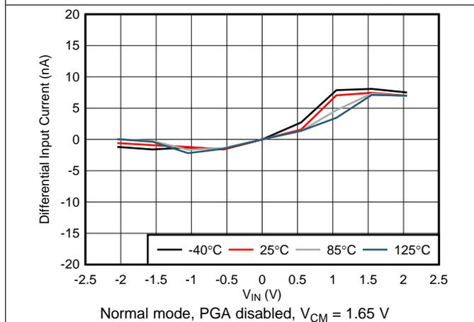
Figure 8. Differential Input Current vs Differential Input Voltage
