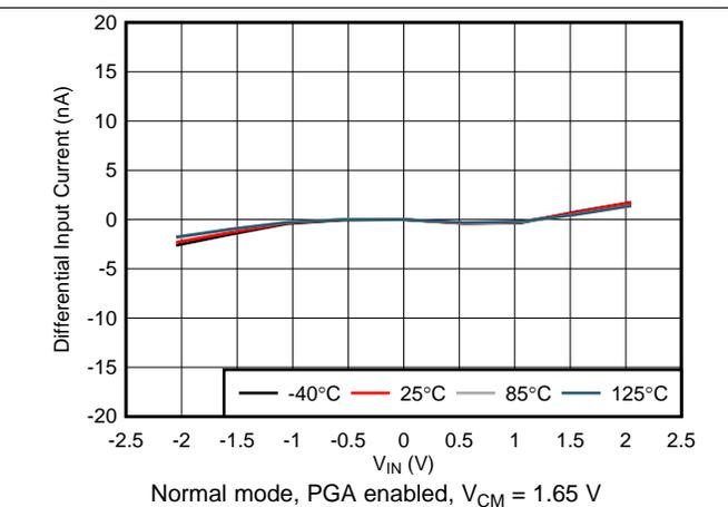
Figure 9. Differential Input Current vs Differential Input Voltage
