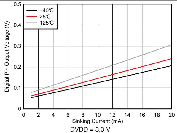
**Figure 35. Digital Pin Output Voltage vs Sinking Current**
