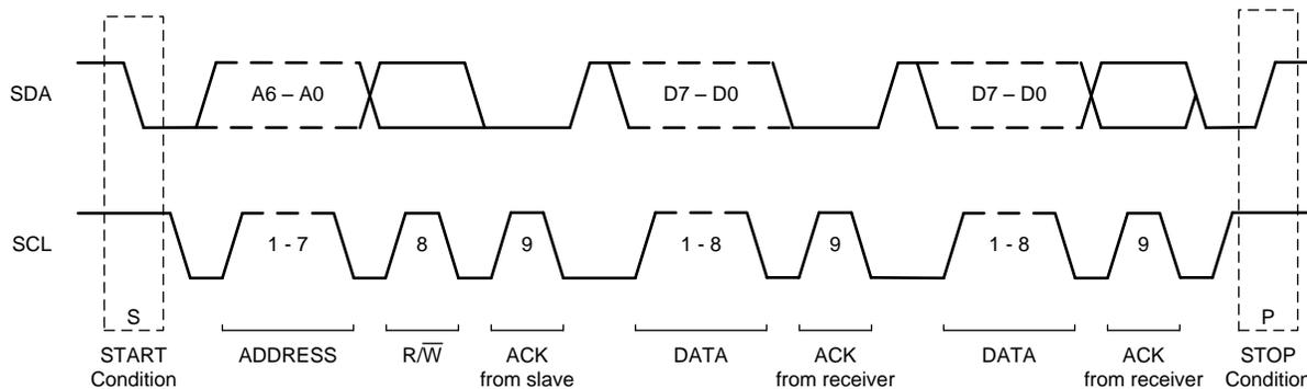
**Figure 55. I<sup>2</sup>C Data Transfer Format**
