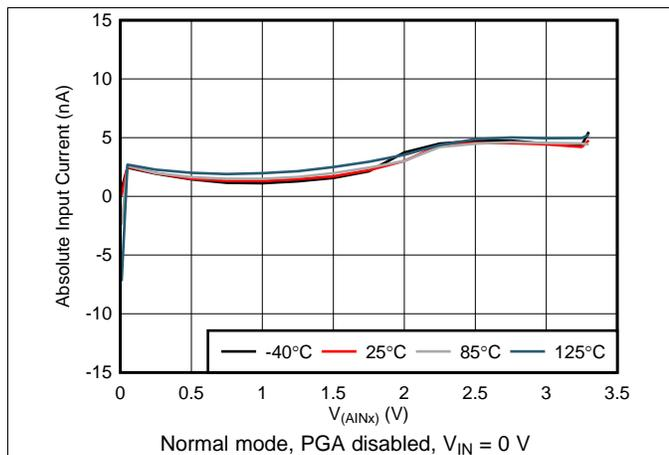
Figure 4. Absolute Input current vs Absolute Input Voltage
