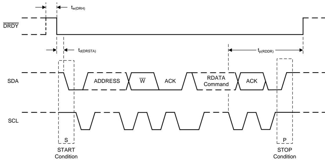
Figure 3.  $\overline{\text{DRDY}}$  Pin Timing Requirements and Switching Characteristics
