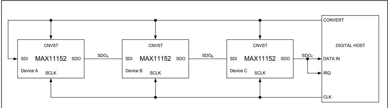
Figure 15. Daisy-Chain Mode with Busy Indicator Connection Diagram
