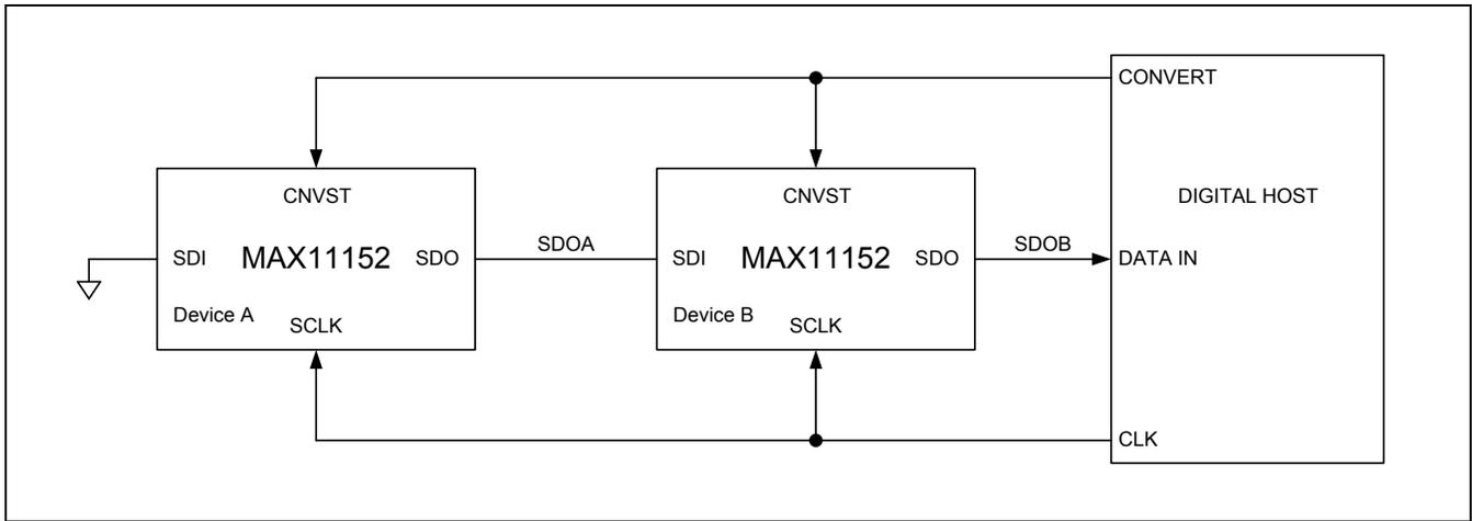
Figure 13. Daisy-Chain, No-Busy Indicator Mode Connection Diagram
