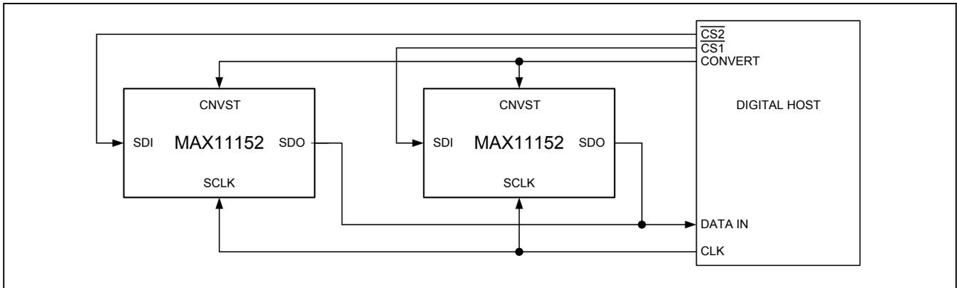
Figure 9.  $\overline{CS}$  Mode 4-Wire, No-Busy Indicator Connection Diagram
