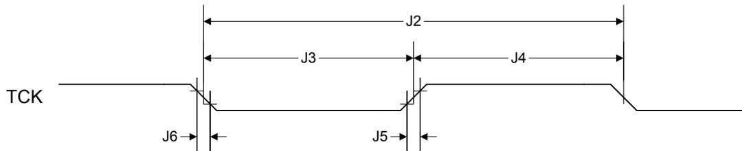
Figure 17-3. JTAG Test Access Port (TAP) Timing
