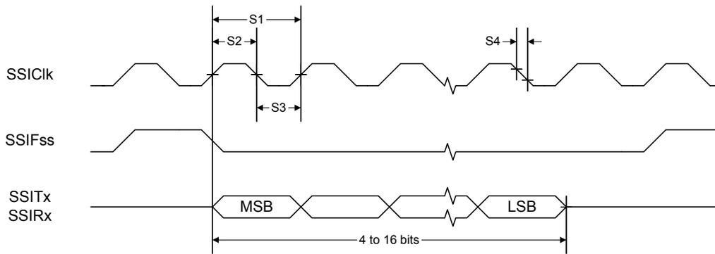
Figure 17-13. SSI Timing for MICROWIRE Frame Format (FRF=10), Single Transfer
