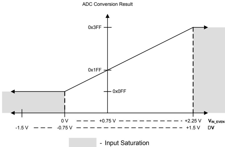
Figure 10-4. Differential Sampling Range,  $V_{IN\_ODD} = 2.25\text{ V}$
