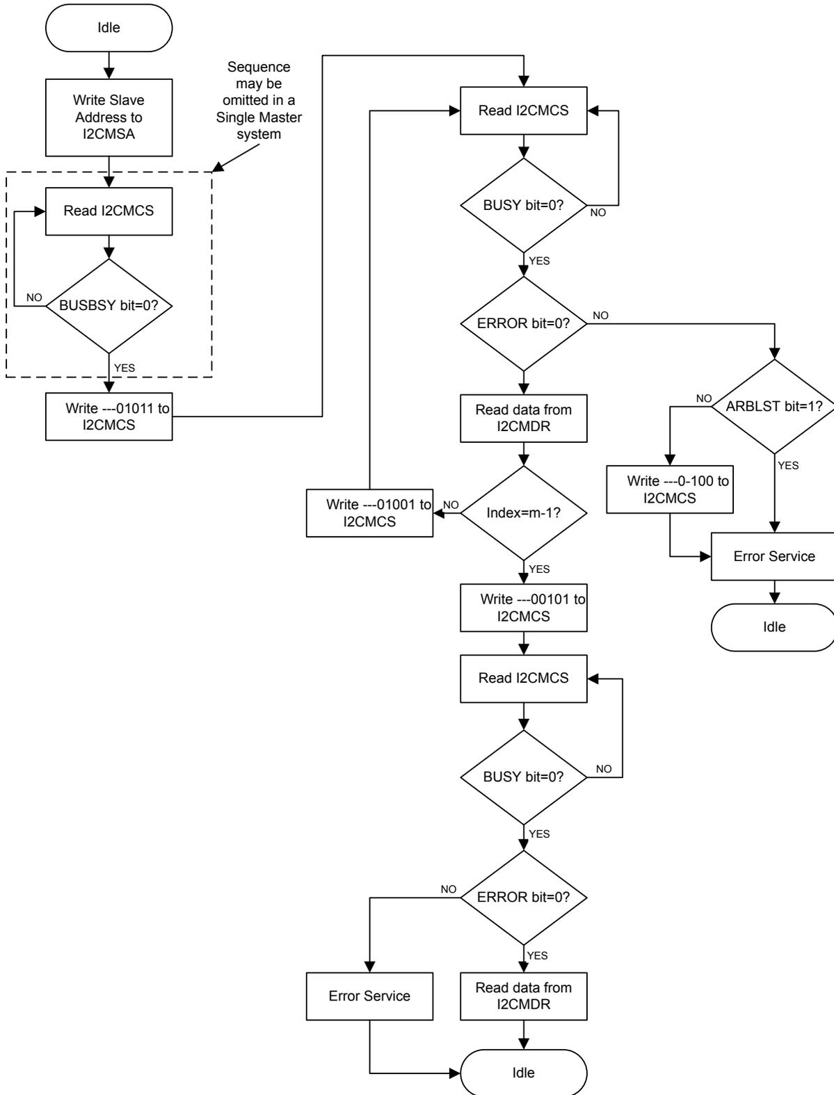
Figure 13-11. Master Burst RECEIVE after Burst SEND
