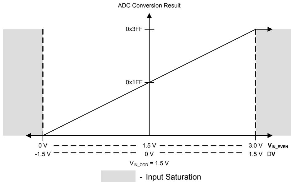
Figure 10-3. Differential Sampling Range,  $V_{IN\_ODD} = 0.75\text{ V}$
