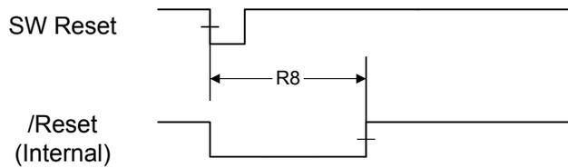
**Figure 17-9. Watchdog Reset Timing**
