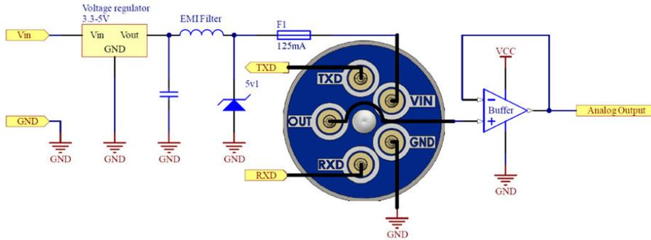
Fig. 1 Example schematic for Interfacing Integrated IR (INIR2-ME5%)
