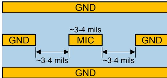
Figure 7. MIC PCB Trace as Shielded Stripline
