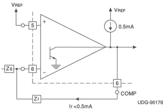
Error Amplifier can source up to 0.5mA.
