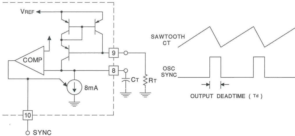
Output deadtime is determined by size of the external capacitor,  $C_T$ , according to the formula:
