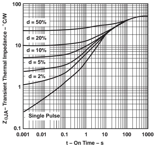
The single-pulse curve represents measured data. The curves for various pulse durations are based on the following equation:
