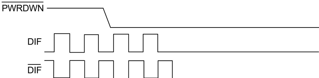
**Figure 1.  $\overline{\text{PWRDN}}$  Assertion**
