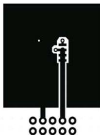
a) 50 °C/W when mounted on a 1 in<sup>2</sup> pad of 2 oz copper.
