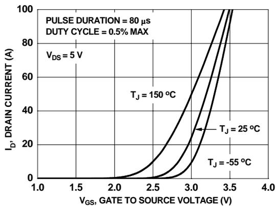
Figure 5. Transfer Characteristics
