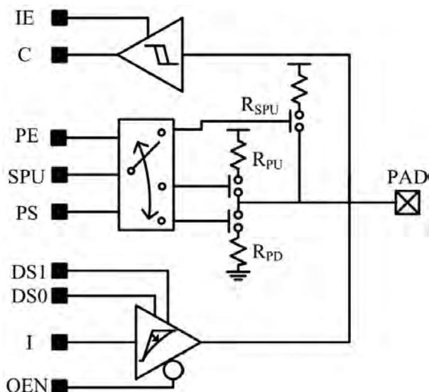
Figure 21. GPIO PAD Block Diagram
