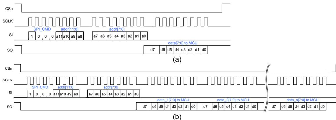
**Figure 17. Register read sequence for (a) a single and (b)  $n$  successive data.**
