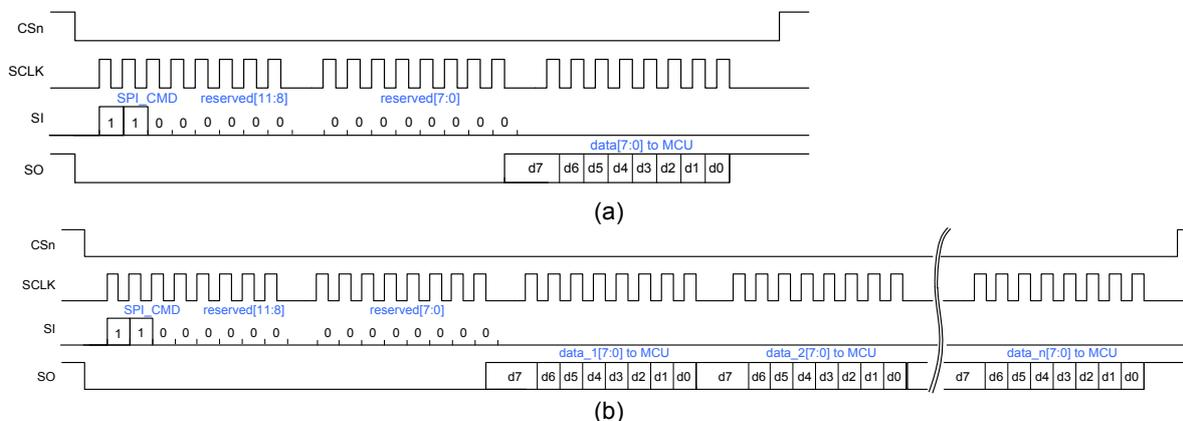
**Figure 19. RX FIFO read sequence. (a) Single and (b) Multiple data access.**
