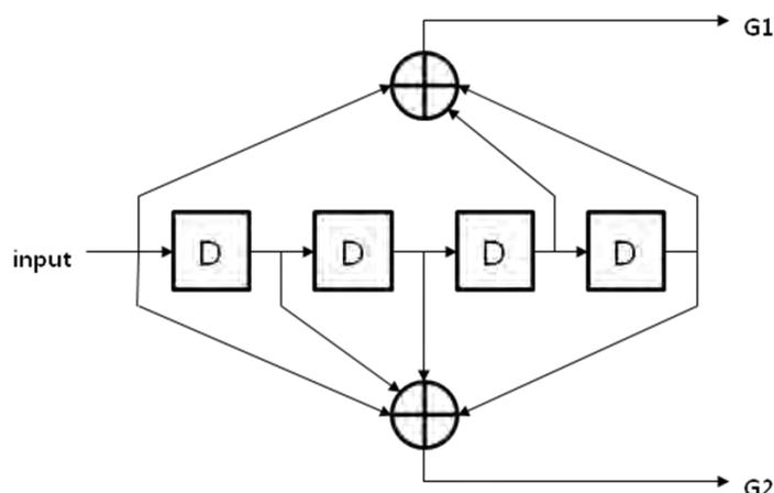
Figure 7. Convolutional encoder with rate of 1/2.
