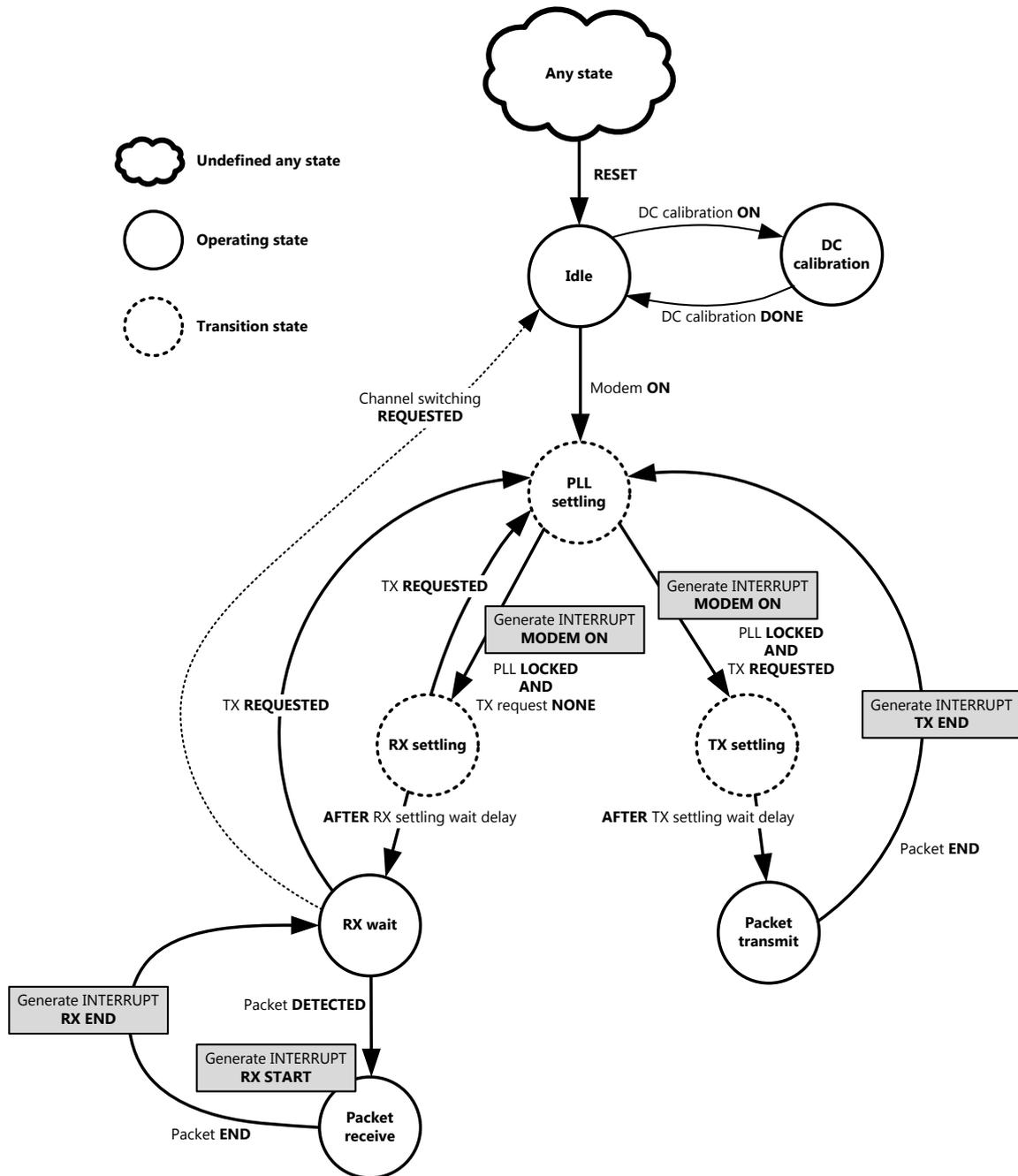
Figure 22. Basic MG2420 State Transition Diagram
