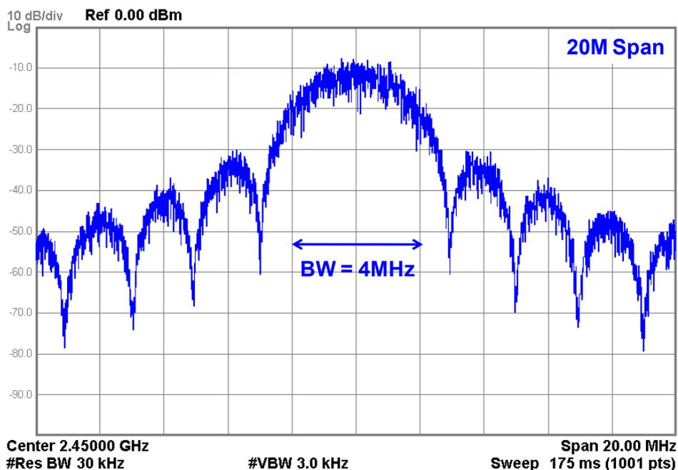
Figure 6. Modulated signal spectrum for 4Mcps mode.
