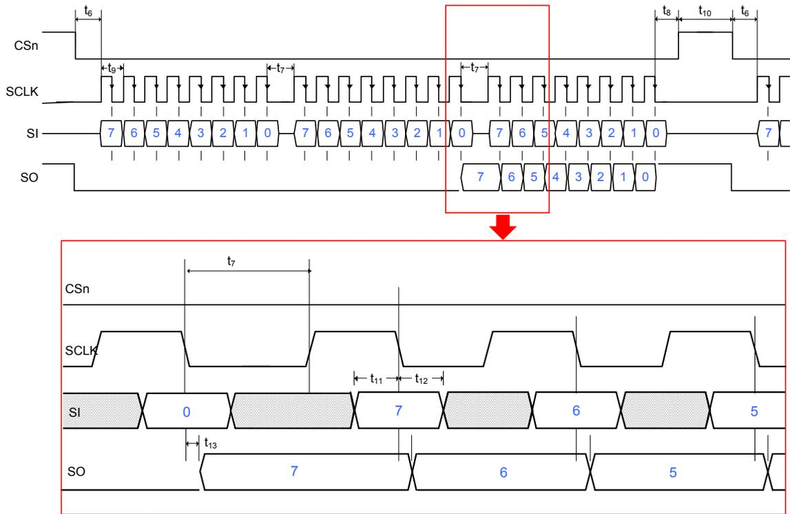
Figure 15. SPI timing diagram.
