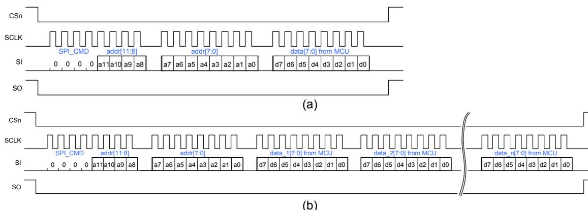
**Figure 16. Register write sequence for (a) a single and (b)  $n$  successive data.**
