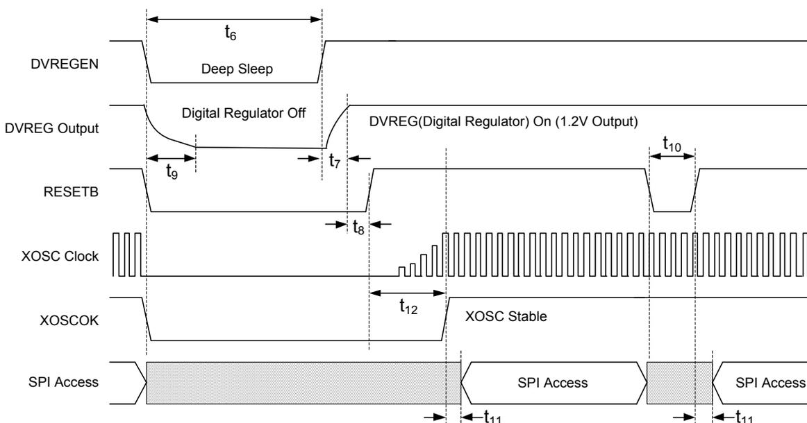
Figure 20. RESETB and DVREGEN signal diagram
