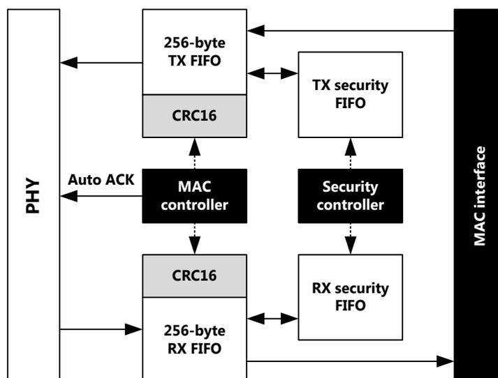
Figure 11. Integrated MAC structure
