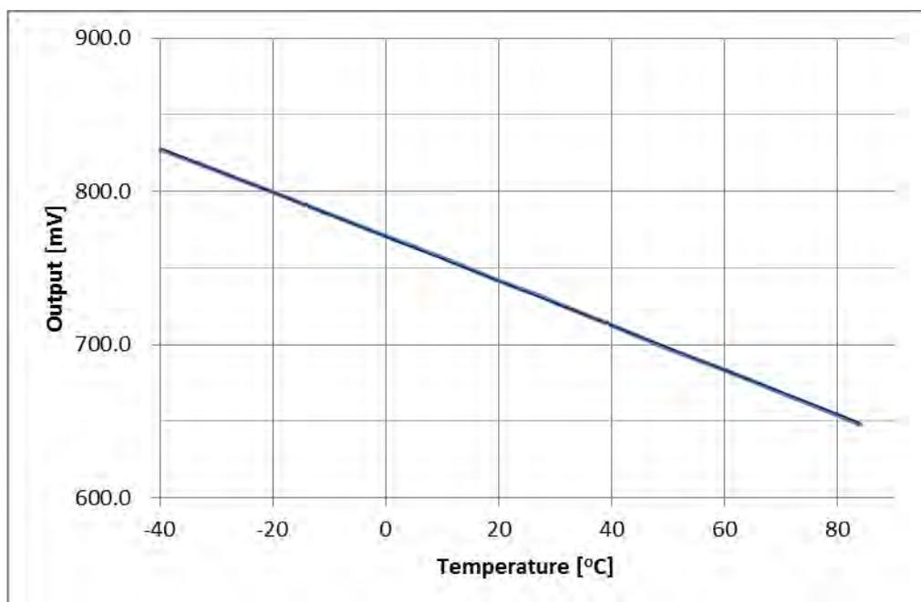
**Figure 13. Temperature sensor output voltage.**
