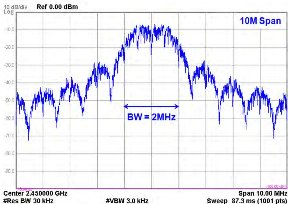
**Figure 5. Modulated signal spectrum for 2Mcps mode.**
