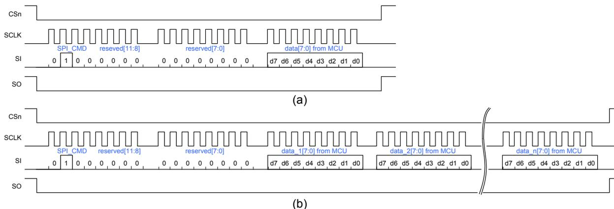
**Figure 18. TX FIFO write sequence. (a) Single and (b) Multiple data access.**
