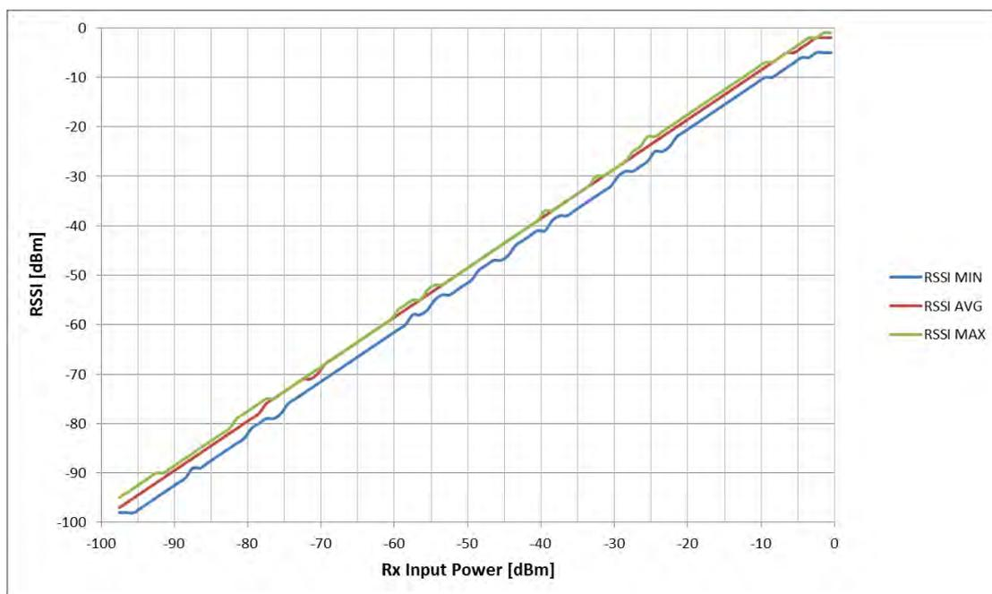
**Figure 10. Typical RSSI value vs. RX input power for 250kbps.**
