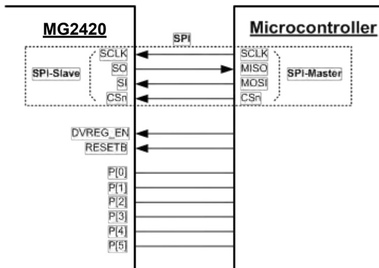
Figure 14. Microcontroller to MG2420 interfaces.
