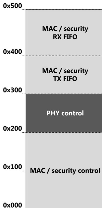
Figure 23. Overall register address space
