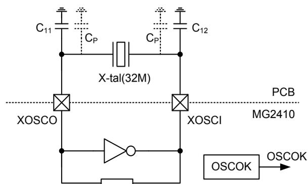
Figure 12. Simplified Crystal Oscillator schematic.
