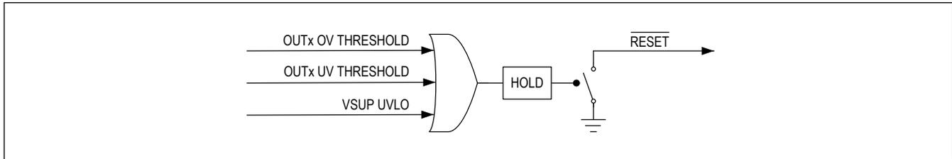
Figure 2. Simplified  $\overline{\text{RESET}}$  Logic Diagram
