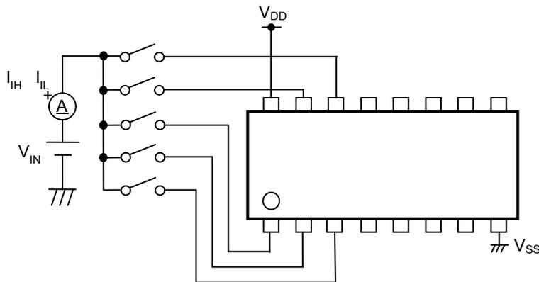
Figure 4. Test Circuit of Input H/L Current
