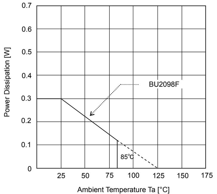
Figure 8. Derating Curve
