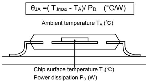
Figure 7. Thermal resistance
