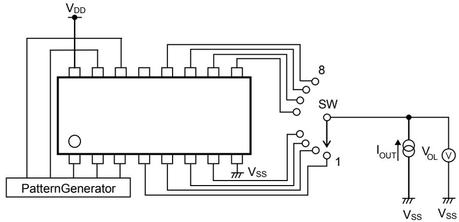
Figure 3. Test Circuit of Output L Voltage
