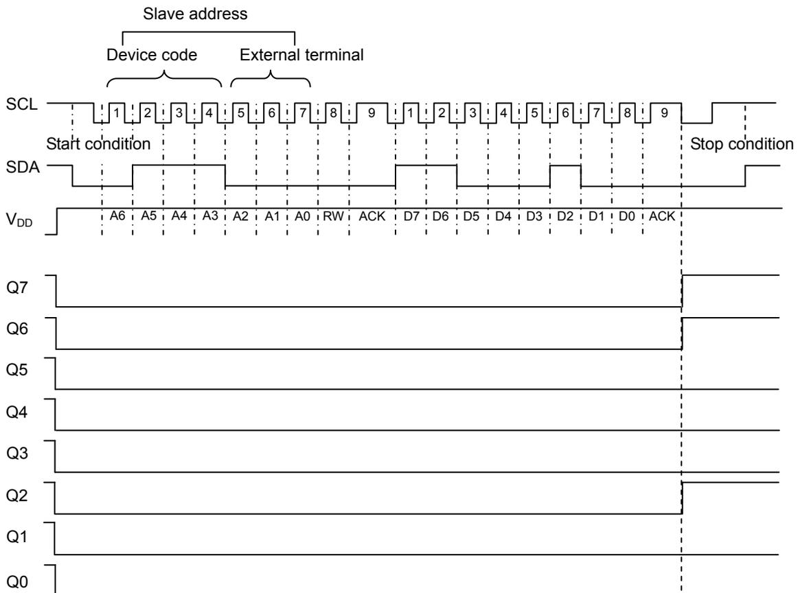
Diagram shows a status where a pull-up resistor is connected to open drain output.
