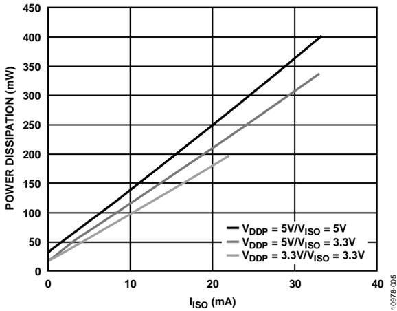
Figure 5. Typical Total Power Dissipation vs.  $I_{ISO}$
