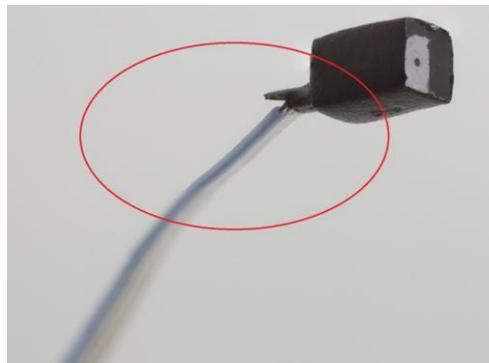
In case the cable is broken in any its other part (non critical area), please refer to section 3. The cable wires have a specific pinout guided by the colored wire (Ground (VSS)). Please be aware that swapping the pinout will cause the camera not to be operational and may cause irreversible damage to the module.
