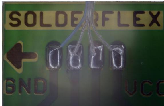
Figure 6 shows an example of the soldered wires on the 4-pin PCB connector, where the VSS/GND wire is on the most-left connector position and VCC is on its most-right.
