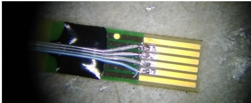
Figure 7 shows an example of the PCB Flex connector, where the colored VSS wire can be easily seen.
