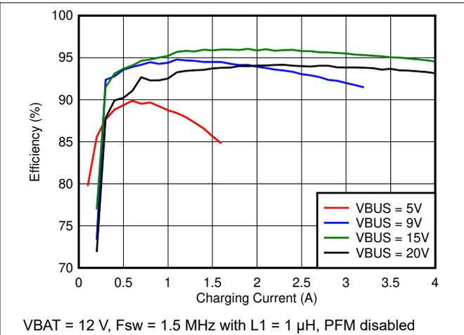
**Figure 7-2. 3s Battery Charge Efficiency vs. Charge Current**
