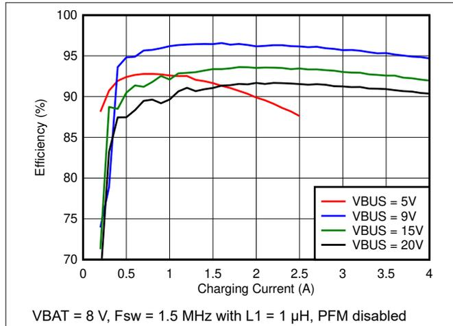
**Figure 7-1. 2s Battery Charge Efficiency vs. Charge Current**
