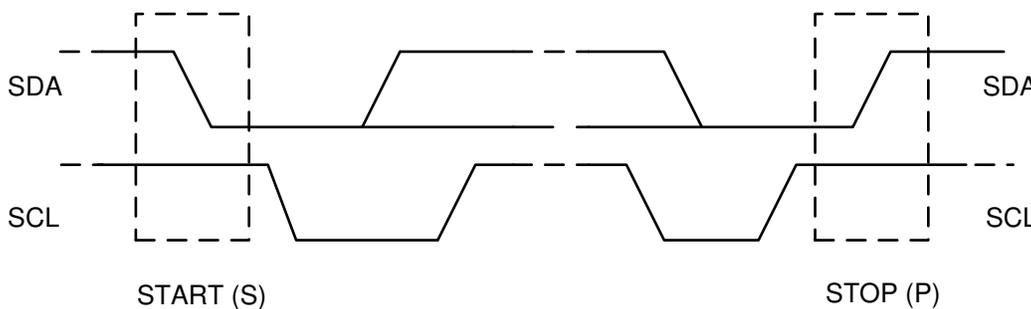
**Figure 8-14. START and STOP Conditions on the I<sup>2</sup>C Bus**
