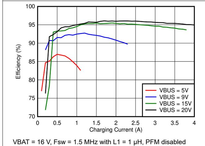
**Figure 7-3. 4s Battery Charge Efficiency vs. Charge Current**
