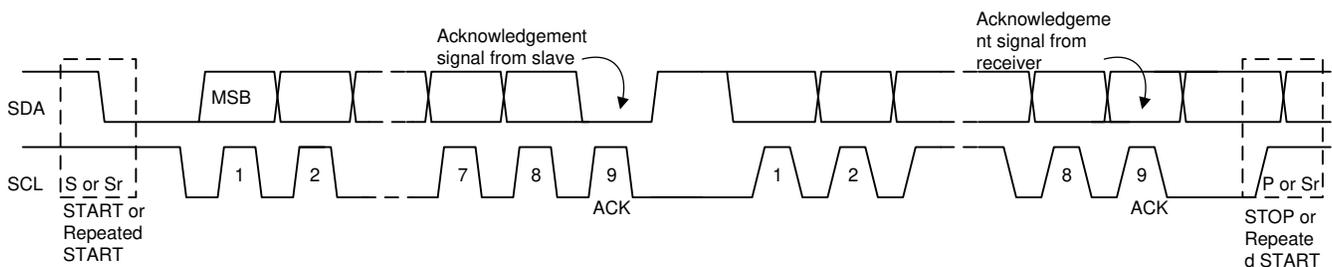
**Figure 8-15. Data Transfer on the I<sup>2</sup>C Bus**
