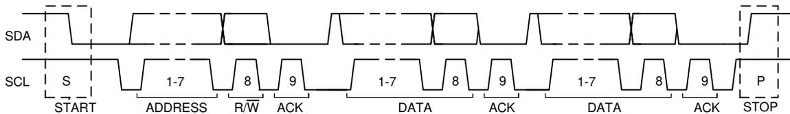
Figure 8-17. Complete Data Transfer on the I<sup>2</sup>C Bus
