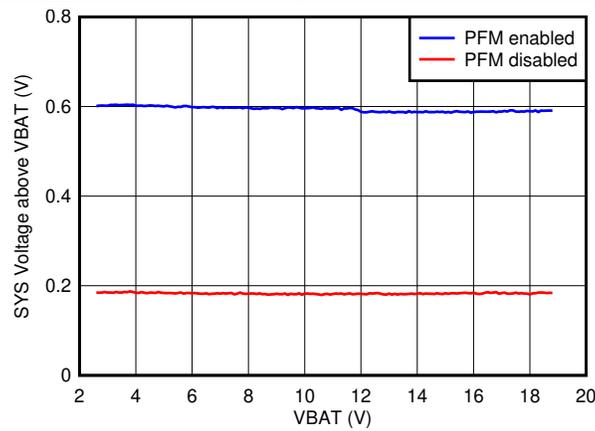
VBUS = 9 V, Fsw = 1.5 MHz with L1 = 1  $\mu$ H, ISYS = 0 A, Charge Disabled
