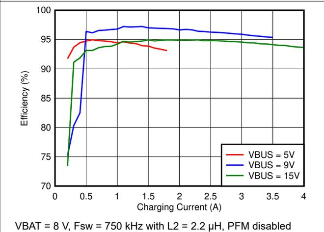
**Figure 7-4. 2s Battery Charge Efficiency vs. Charge Current**
