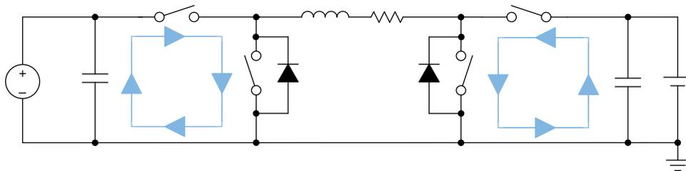
**Figure 11-1. Buck-Boost Converter High Frequency Current Path**
