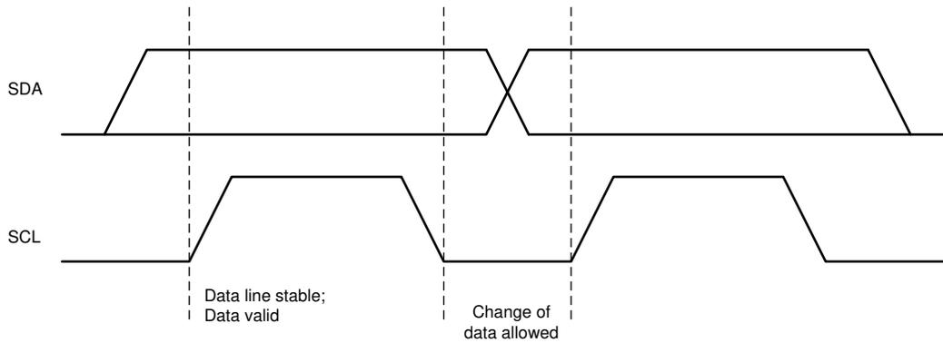
**Figure 8-13. Bit Transfers on the I<sup>2</sup>C Bus**
