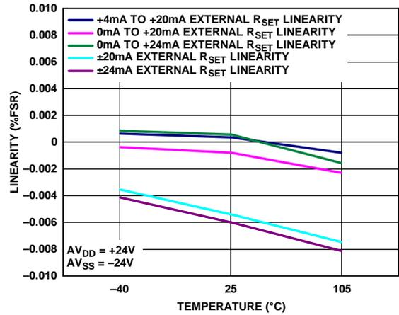
Figure 33. INL vs. Temperature, External R<sub>SET</sub> Sense Resistor
