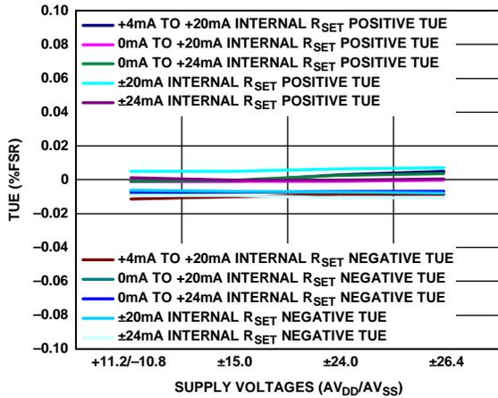
Figure 31. Total Unadjusted Error (TUE), Current Mode, Internal R<sub>SET</sub> Sense Resistor
