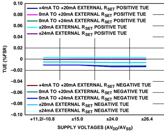
Figure 30. Total Unadjusted Error (TUE), Current Mode, External R<sub>SET</sub> Sense Resistor
