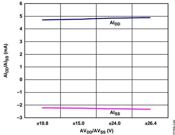
Figure 49. A<sub>I\_DD</sub>/A<sub>I\_SS</sub> vs. AV<sub>DD</sub>/AV<sub>SS</sub>, V<sub>OUT</sub> = 0 V
