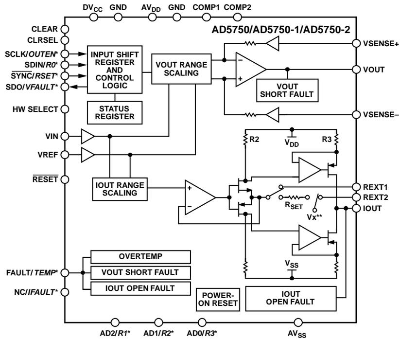
\* DENOTES SHARED PIN. SOFTWARE MODE DENOTED BY REGULAR TEXT, HARDWARE MODE DENOTED BY *ITALIC* TEXT. FOR EXAMPLE, FOR FAULT/ *TEMP* PIN, IN SOFTWARE MODE, THIS PIN TAKES ON FAULT FUNCTION. IN HARDWARE MODE, THIS PIN TAKES ON *TEMP* FUNCTION.
