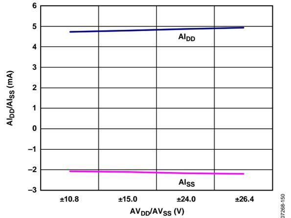
Figure 50. A<sub>I\_DD</sub>/A<sub>I\_SS</sub> vs. AV<sub>DD</sub>/AV<sub>SS</sub>, I<sub>OUT</sub> = 0 mA
