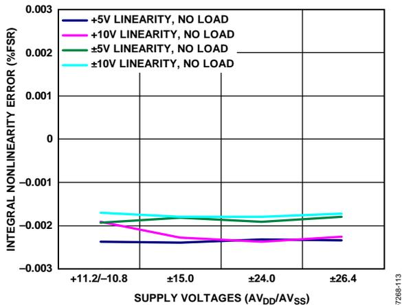
Figure 13. Integral Nonlinearity Error vs. Supply Voltage
