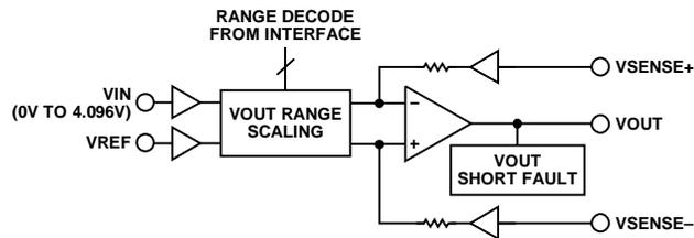
Figure 54. Voltage Output
