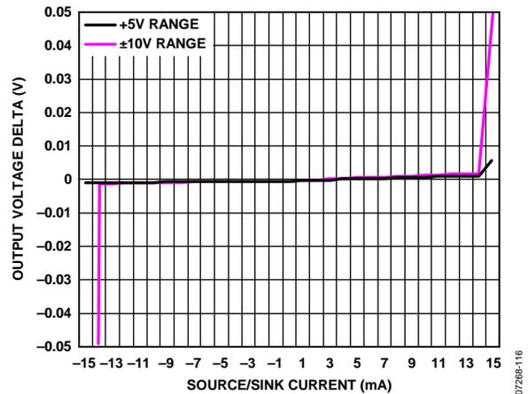
Figure 16. Source and Sink Capability of Output Amplifier
