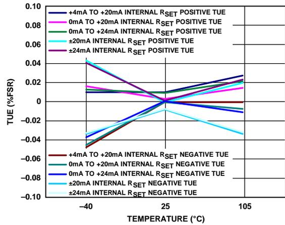
Figure 34. Total Unadjusted Error (TUE) vs. Temperature, Internal R<sub>SET</sub> Sense Resistor
