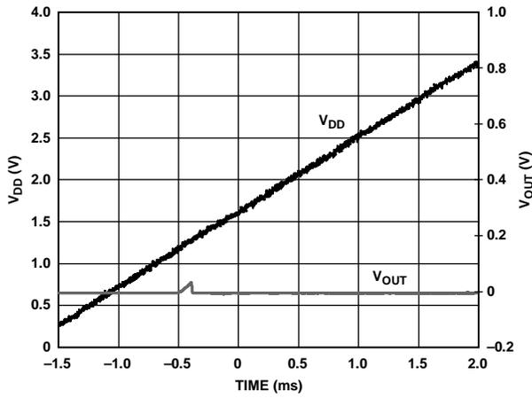
Figure 23. V<sub>DD</sub> and V<sub>OUT</sub> vs. Time on Power-Up
