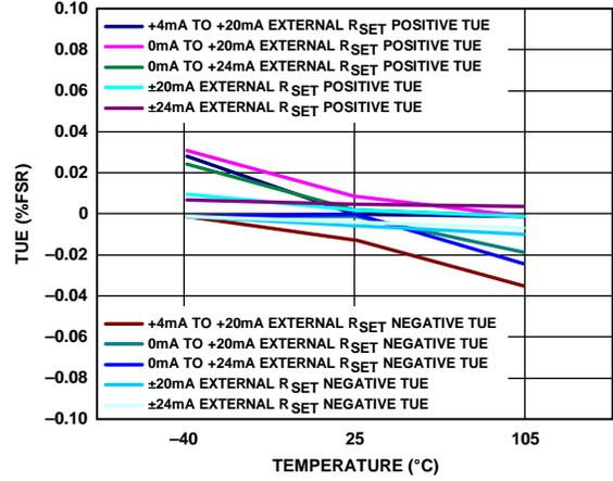
Figure 35. Total Unadjusted Error (TUE) vs. Temperature, External R<sub>SET</sub> Sense Resistor
