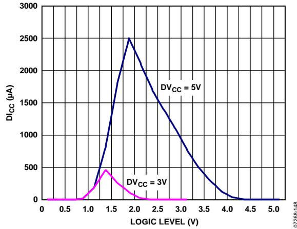
Figure 48. D<sub>Icc</sub> vs. Logic Input Voltage
