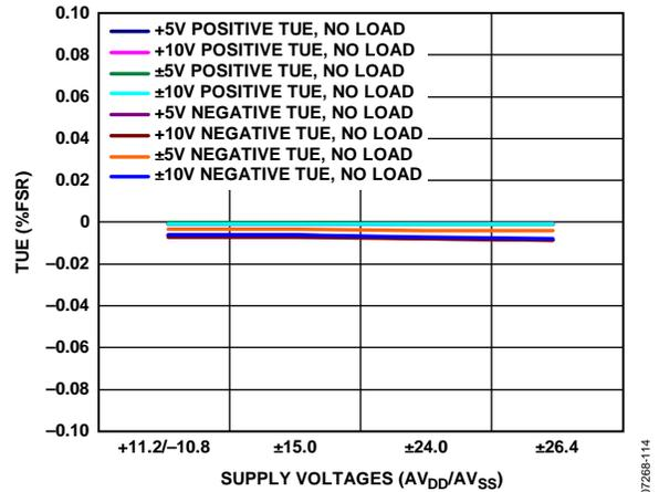
Figure 14. Total Unadjusted Error (TUE) vs. Supply Voltages
