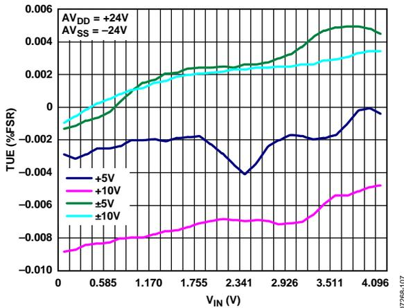
Figure 7. Total Unadjusted Error (TUE) vs.  $V_{IN}$
