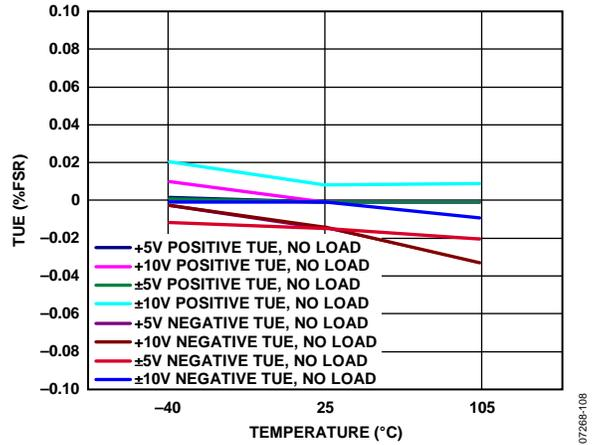
Figure 8. Total Unadjusted Error (TUE) vs. Temperature
