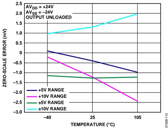
Figure 12. Zero-Scale Error (Offset Error) vs. Temperature
