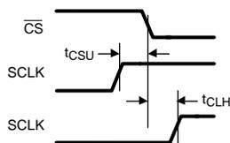
Figure 4. SCLK and CS Timing Parameters
