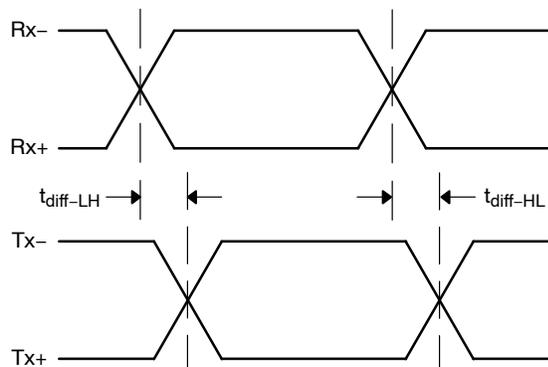
Figure 3. Propagation Delay
