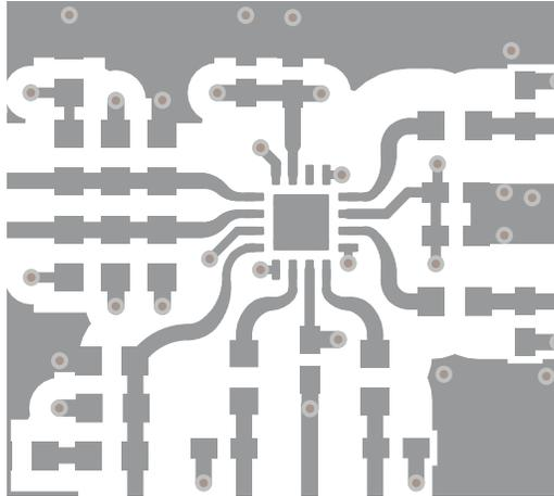
**Figure 16. General PCB Ground Layout for Thermal Reliability**
