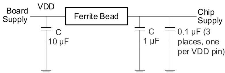
**Figure 15. Power-Supply Decoupling**
