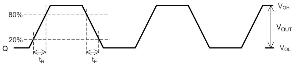
Figure 6. Output Voltage, and Rise and Fall Times
