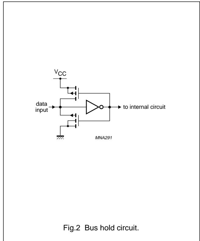
Fig.2 Bus hold circuit.
