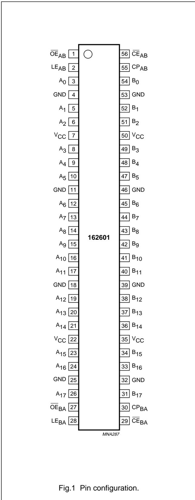
Fig.1 Pin configuration.
