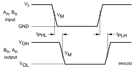
Fig.6 The input  $A_n$ ,  $B_n$  to output  $B_n$ ,  $A_n$  propagation delay times.
