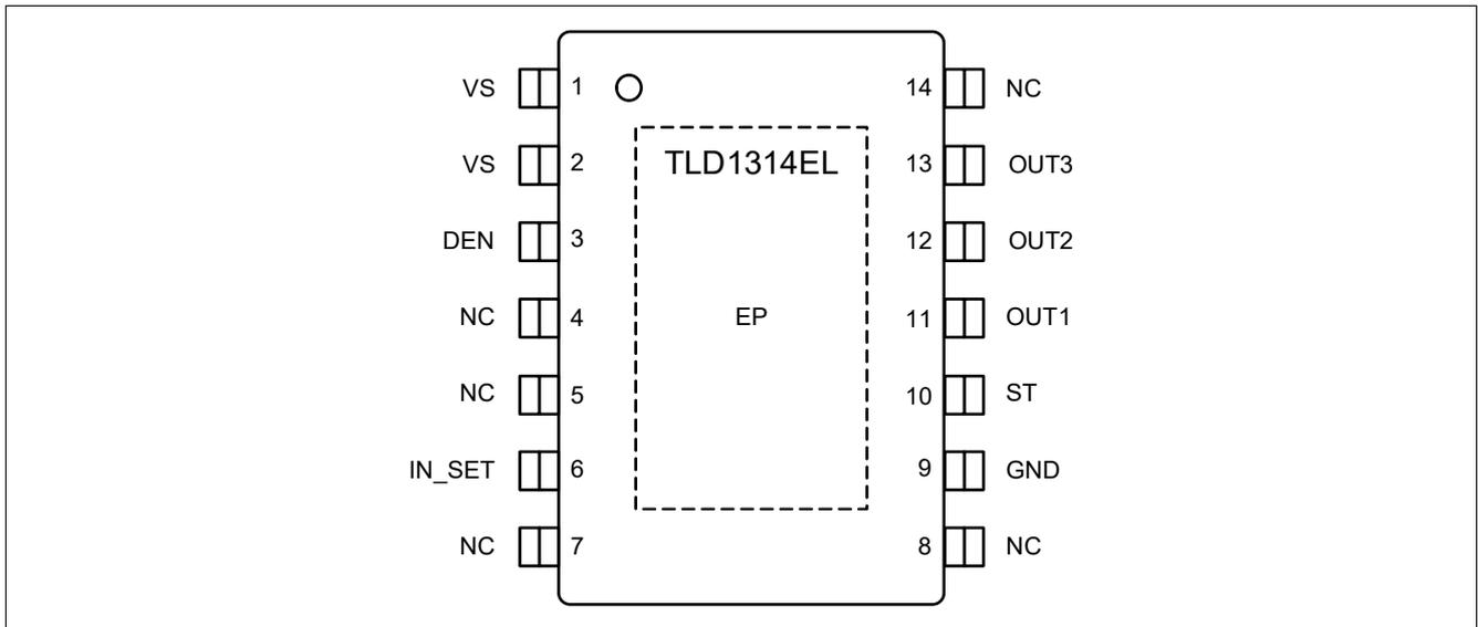
Figure 2 Pin Configuration
