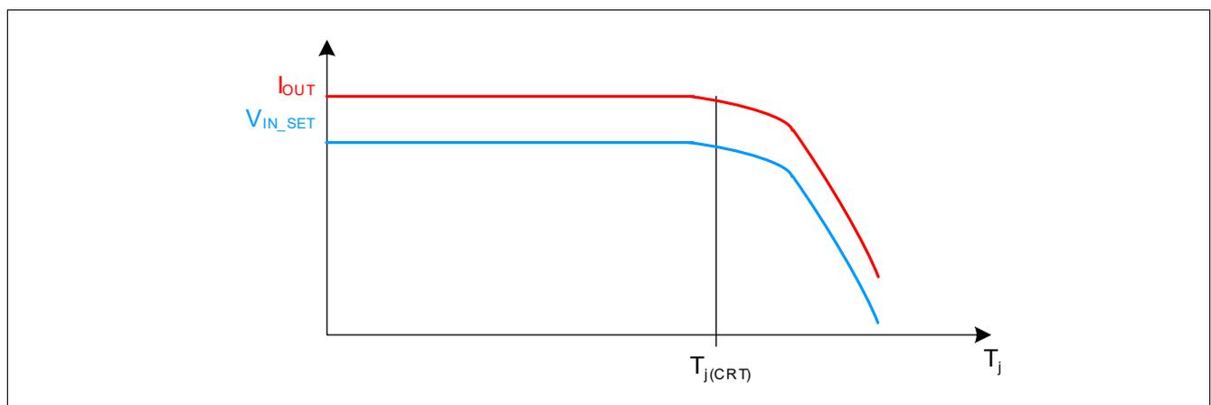
**Figure 18 Output current reduction at high temperature**
