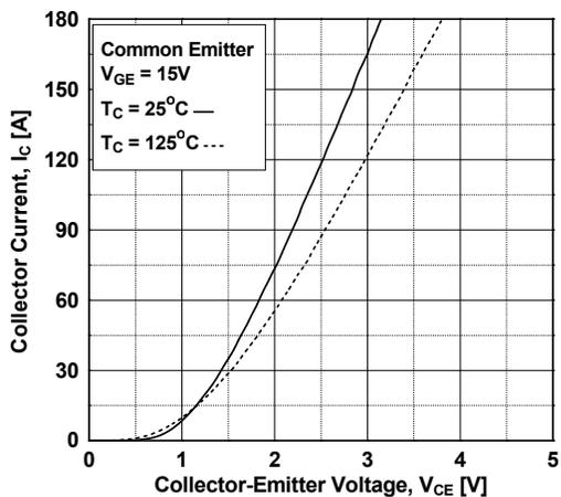
Figure 4. Transfer Characteristics
