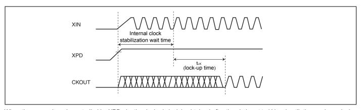
When the power down is controlled by XPD pin, the desired clock is obtained after the pin is set to H level until the maximum lock-up time  $t_{LK}$  is elapsed.
