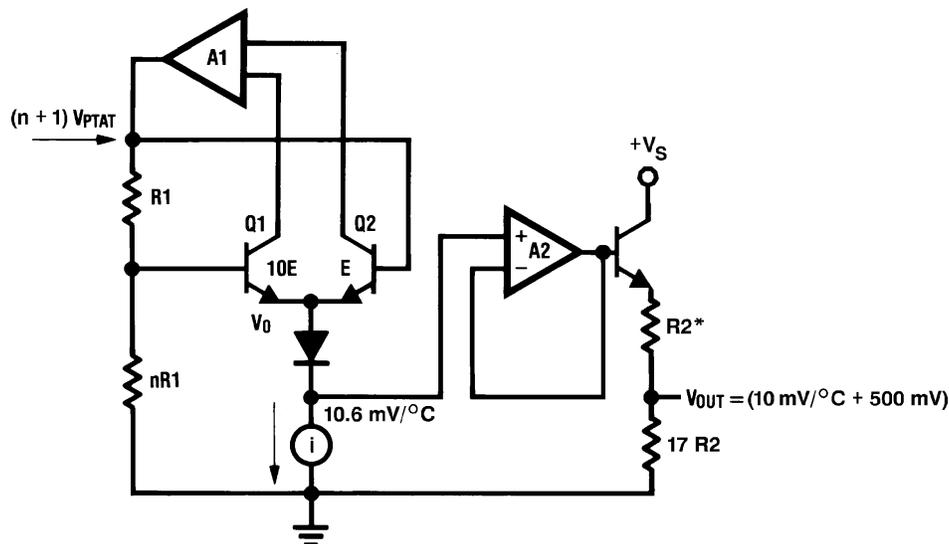
\*R2  $\approx$  2k With a typical  $1300\text{ ppm}/^{\circ}\text{C}$  Drift.
