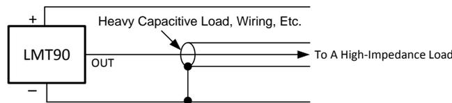
Figure 12. LMT90 No Decoupling Required for Capacitive Load
