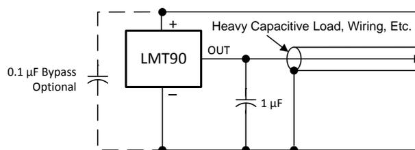
Figure 13. LMT90 With Filter for Noisy Environment
