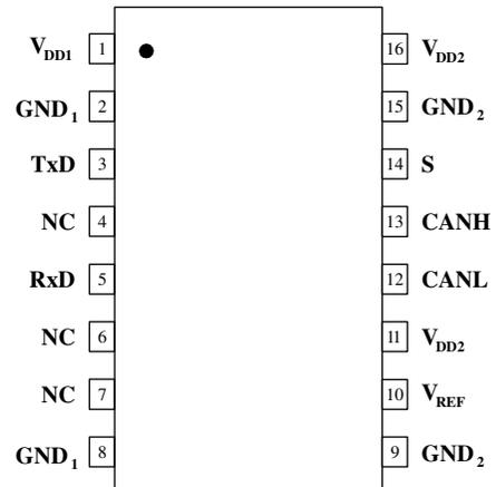
\*Pin 11 is not internally connected to pin 16; both should be connected to the V<sub>DD2</sub> power supply for normal operation.
