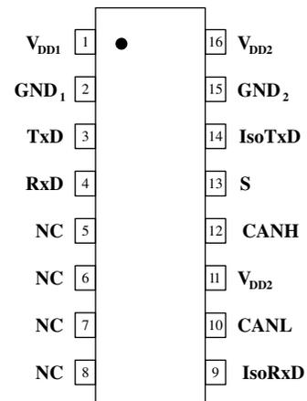
\*Pin 11 is not internally connected to pin 16; both should be connected to the V<sub>DD2</sub> power supply for normal operation.
