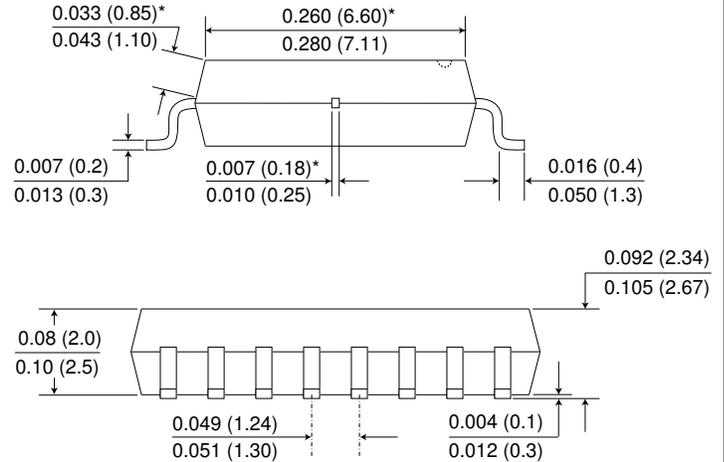
NOTE: Pin spacing is a BASIC dimension; tolerances do not accumulate
