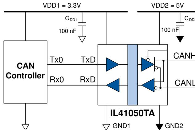
Figure 3. Isolated CAN node using the IL41050TA.
