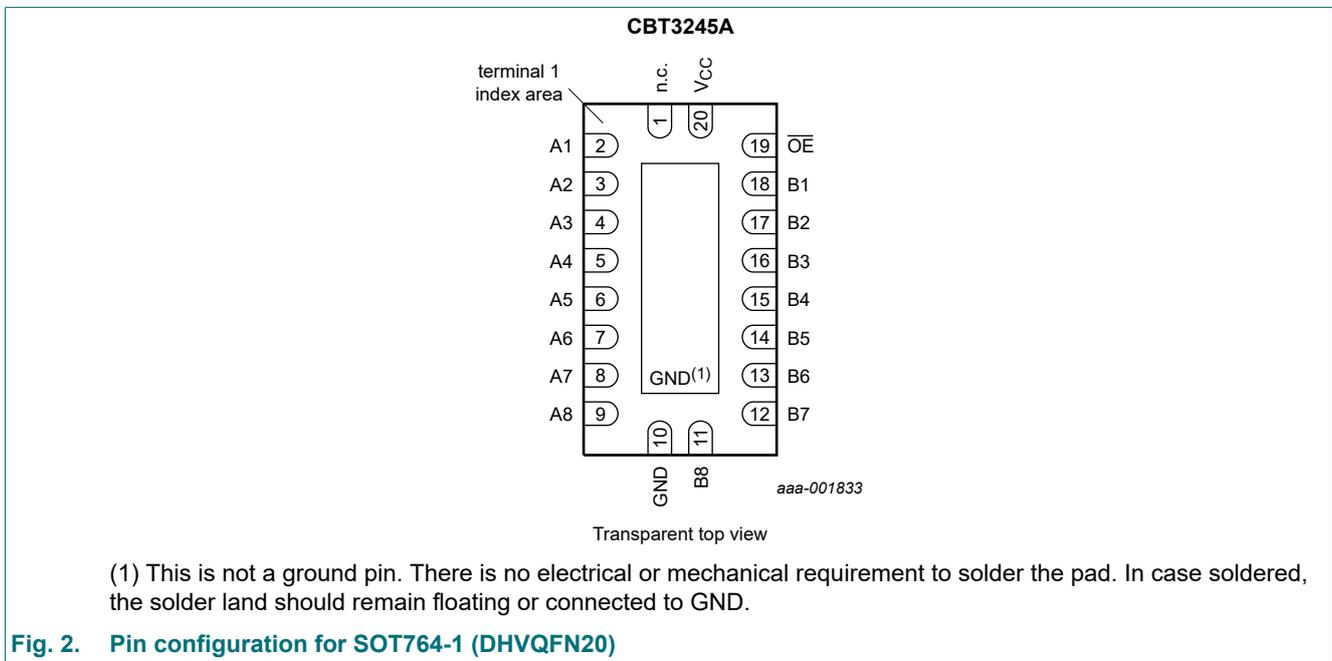
Fig. 2. Pin configuration for SOT764-1 (DHVQFN20)
