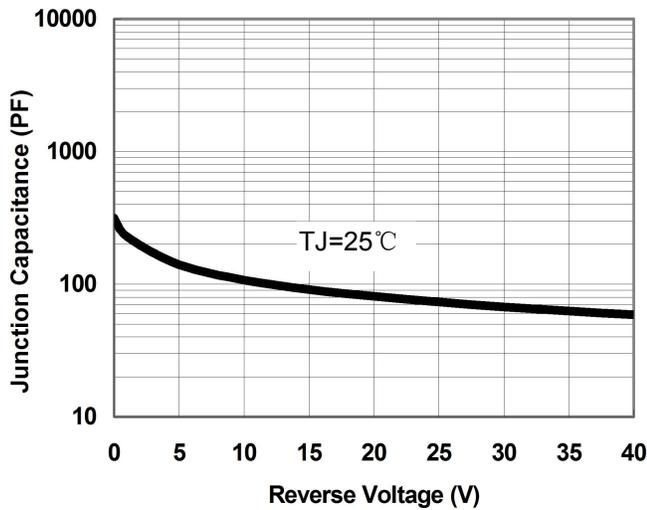
Fig.1-Typical Junction Capacitance
