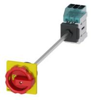
Load disconnector 3LD3, lu 63 A Main switch 3-pole Rated operating capacity at AC-23 A at 400V 22.0 kW floor mounting Basic switch with door coupling Central hole mounting 22.5mm Rotary actuator red / yellow 66 x 66 mm
