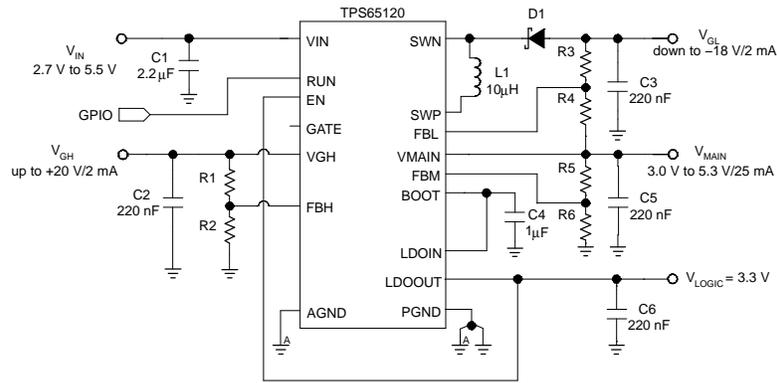
Figure 23. Complete TFT-LCD Power Supply from 1 cell Li-Ion
