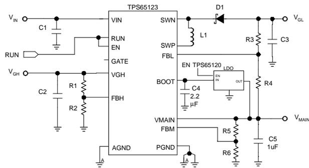
**Figure 28. Boosting Main Output Current,  $I_{MAIN} > 25mA$**
