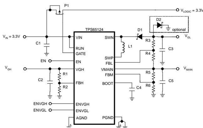
Figure 20. Power Sequencing on Digital Supply Voltage,  $V_{LOGIC}$
