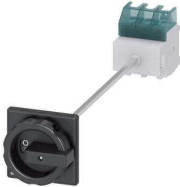
SENTRON, Switch disconnecter 3LD, main switch, 3-pole, Iu: 63 A, Operating power / at AC-23 A at 400 V: 22 kW, floor mounting with door coupling, rotary operating mechanism, black, 4-hole mounting of the handle
