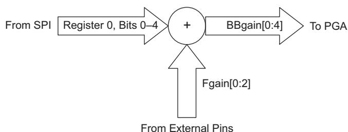
**Figure 33. PGA Gain Control Word**
