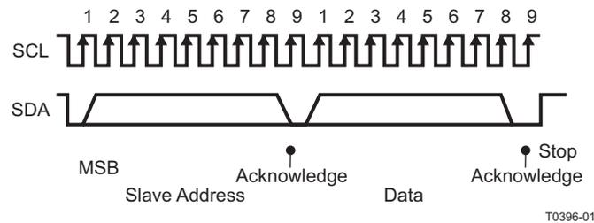
Figure 51. I<sup>2</sup>C Address, Data Cycle(s), and Stop
