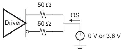
Figure 16. TMDS Main Link Short-Circuit Output Circuit
