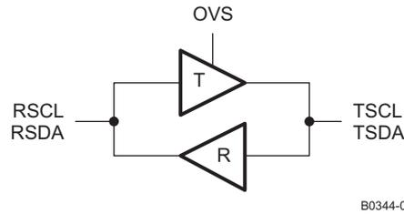
**Figure 40. I<sup>2</sup>C Drivers in the TMDS361B (R Side Is the HDMI Source Side, T Side Is the HDMI Sink Side)**
