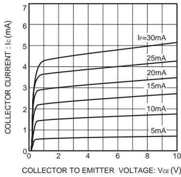
Fig.10 Output characteristics
